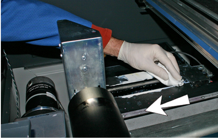
Figure 10 Cleaning the top of the service station
