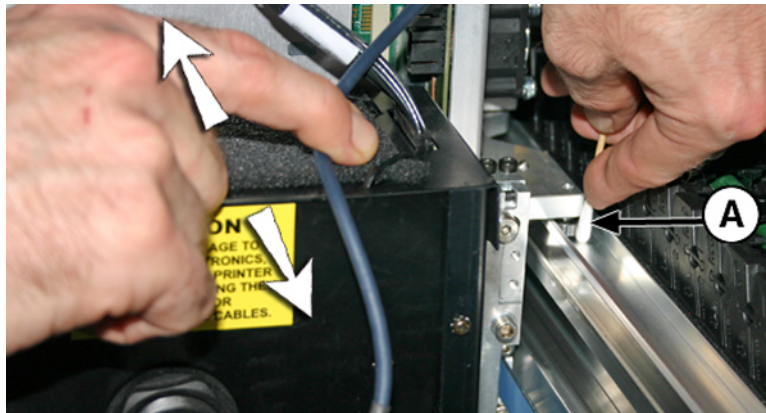
Figure 15 Cleaning carriage-wheel with cotton swab
