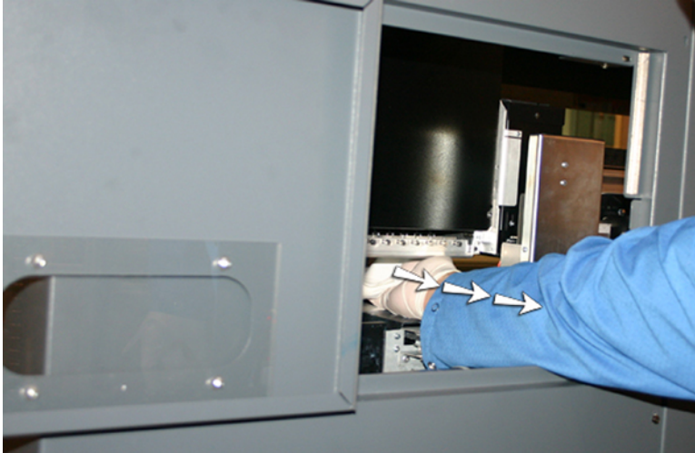
Figure 5 Reaching the printheads through the access door
