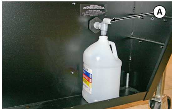
Figure 10-24 Waste ink bottle and spigot
