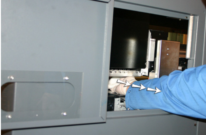
Figure 10-5 Reaching the printheads through the access door
