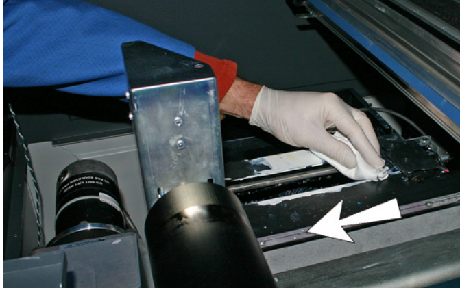
Figure 10-10 Cleaning the top of the service station
