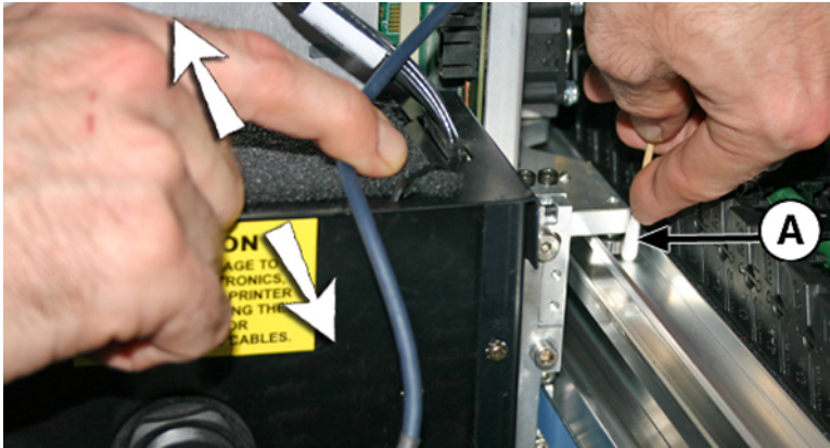
Figure 10-15 Cleaning carriage-wheel with cotton swab
