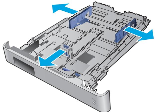
3. To load legal-size paper, extend the tray front by pressing the blue latch and pulling the front of the tray.
