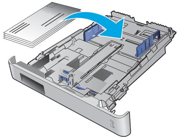
4. Make sure that the envelope stack is flat at all four corners. Slide the length and width guides so that they are against the stack.
