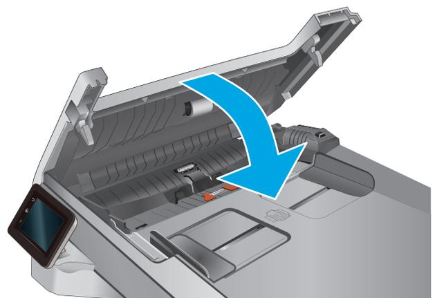
4. Lift the document feeder input tray to provide better access to the document feeder output bin, and then remove any jammed paper from the output area.
