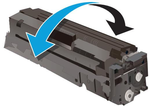
7. Do not touch the imaging drum on the bottom of the toner cartridge. Fingerprints on the imaging drum can cause print-quality problems.
