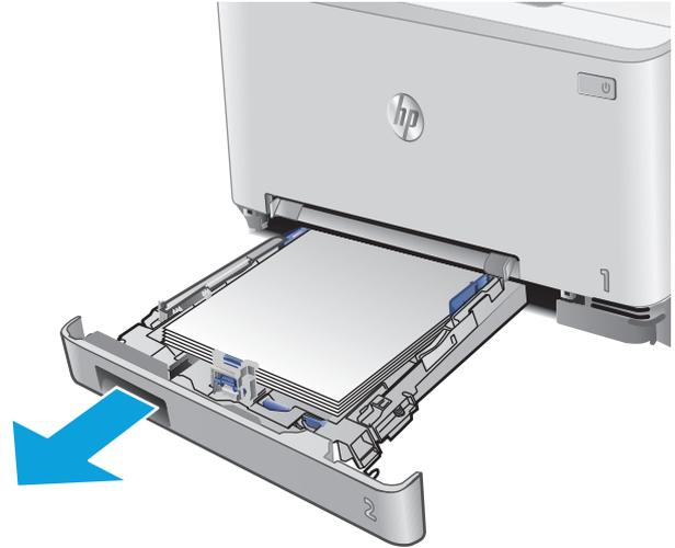
2. Push down on the single-sheet priority feed slot, and then pull out the feed slot tray.
