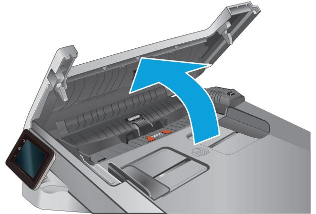
2. Use a moist, lint-free cloth to wipe both pickup rollers and the separation pad to remove dirt.
