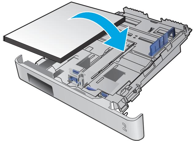
5. Make sure that the paper stack is flat at all four corners. Slide the paper length and width guides so that they are against the stack of paper.
