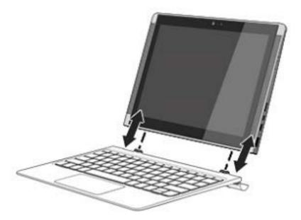
• To remove the tablet from the keyboard base, lift one corner (1) of the tablet to release it.
