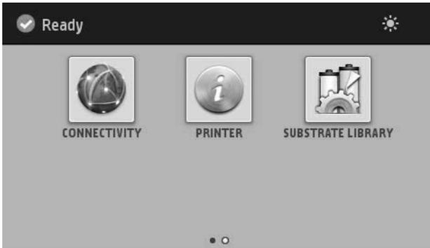
The front panel has a large central area to display dynamic information and icons. On the left and right sides you can see up to four fixed icons at different times. Normally they are not all displayed at the same time.
