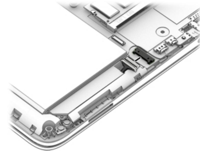
2. Disconnect the subwoofer cable **(1)** from the system board.
