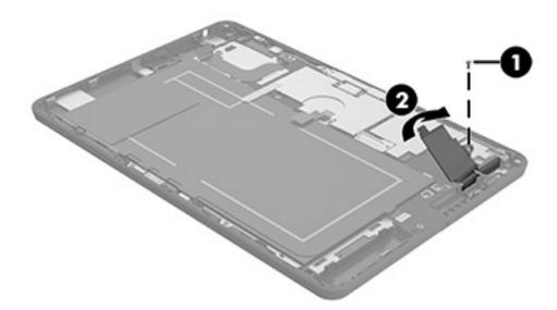
Remove the two 1.2 mm PO Phillips screws that secure the POGO pin metal bracket to the system board and the two 1.2 mm PO Phillips-head screws that secure the display panel cable bracket, and then remove the brackets (1). 3. Disconnect the POGO pin connector (2) from the system board and disconnect the microphone ribbon cable, and disconnect the right speaker cable (3) and move the cables out of the way.
