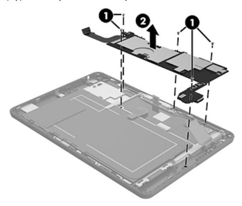
7. Turn over the system board, and then release the ZIF connector to remove the audio cable (1) from the system board.
