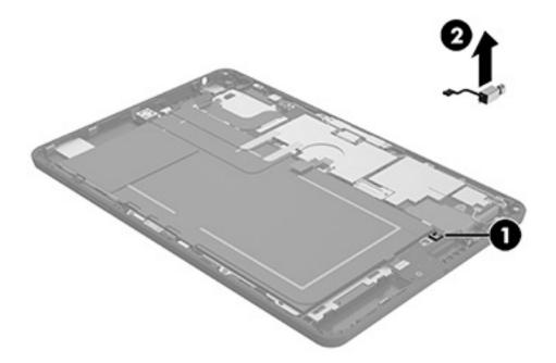
Reverse this procedure to install the vibration motor board.
