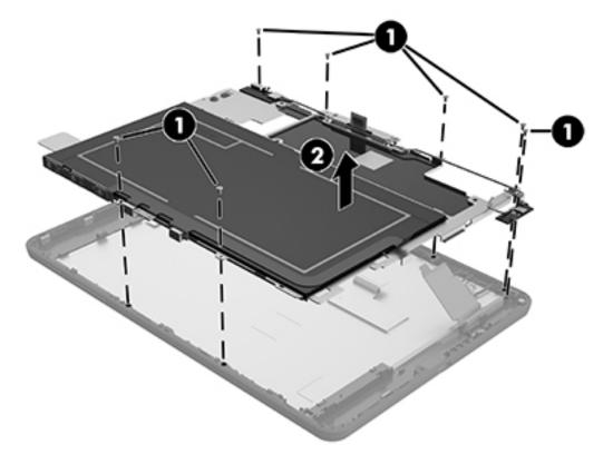
Reverse this procedure to install the battery and middle plate.
