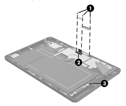
Carefully disconnect the wireless LAN antenna cables (1) from the system board, Remove the MAIN wireless LAN antenna cable from the routing clips on the system board and remove the cable (2).
