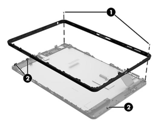
Reverse this procedure to install the outer ring.
