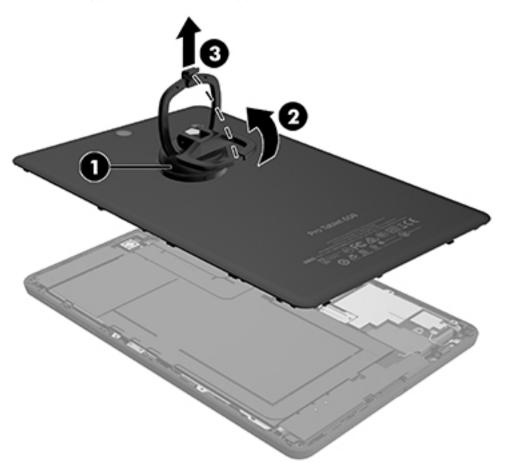
Reverse this procedure to install the back cover.
