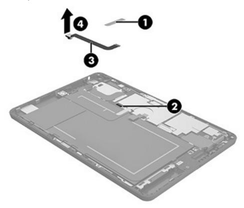
Reverse this procedure to install the front-facing webcamera.
