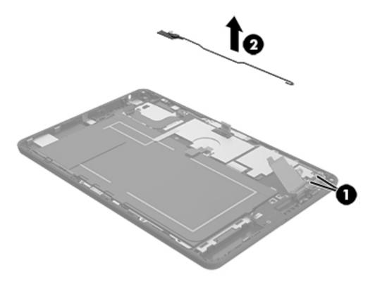
Remove the five Phillips silver screws (1) securing the system board to the display panel assembly.
