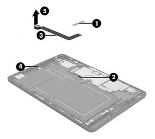
Reverse this procedure to install the rear-facing webcamera.
