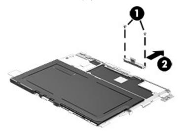
Reverse this procedure to install the POGO pin connector.
