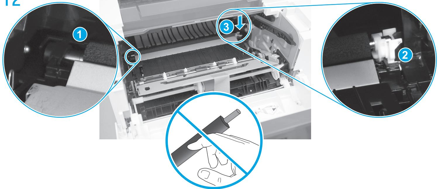
**EN** Place the left (shaft) end of the roller in the holder (callout 1), lower the right end (with the clip) into place making sure that the clip and spring are aligned (callout 2), and then push down (callout 3) on the clip until it snaps in place.
