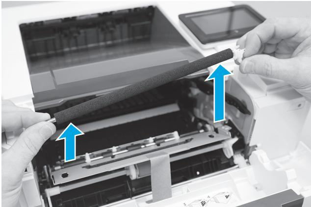
**EN** Remove the transfer roller from the printer.
