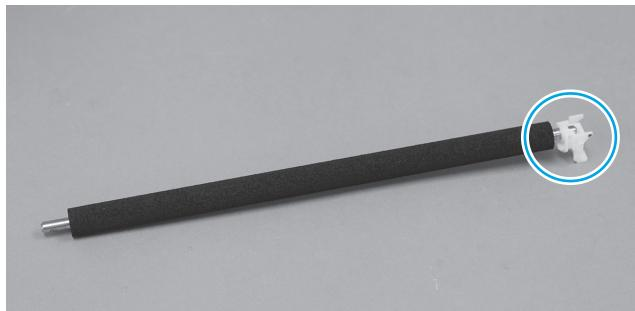
**EN** Install the clip (from step 8) on either end of the replacement transfer roller.
