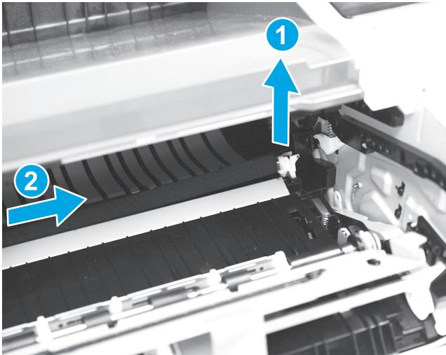
**EN** Grasp the silver shaft end of the roller or the white retainer clip, raise the right-end of the roller up, and then slide the roller to the right to release the left-end of the roller shaft.
