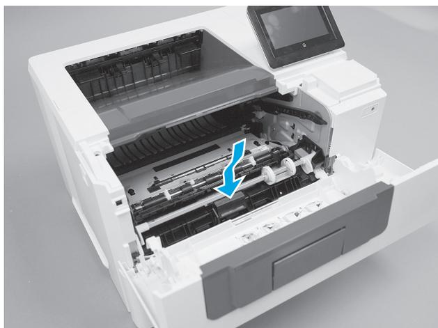
**EN** Install the pad assembly into the holder.
