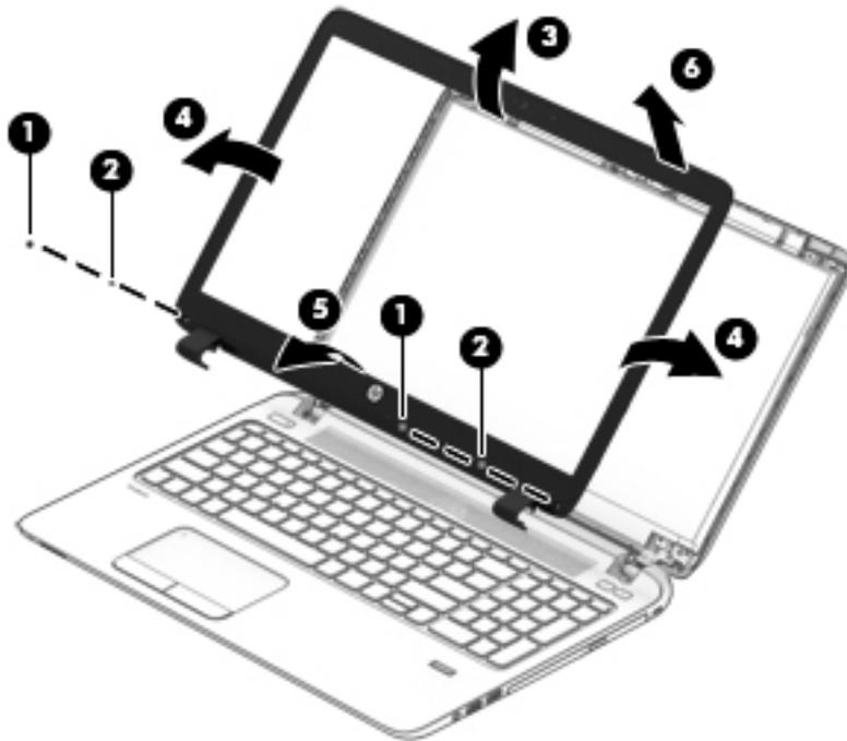
**7. If it is necessary to replace the webcam or microphone module, gently pull the module away from the double-sided tape on the display enclosure (1), and then disconnect the cable from the module (2).**
