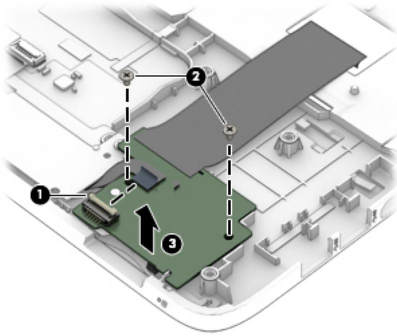
Reverse this procedure to install the card reader board.
