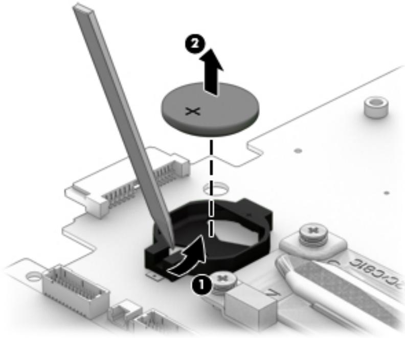
Reverse this procedure to install the RTC battery.
