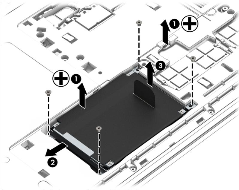
4. To remove the hard drive cover and bracket from the hard drive, lift the Mylar cover up off the drive **(1)**, remove the 4 Phillips PM3.0x3.0 screws **(2)** that secure the bracket to the drive, and then lift the bracket up and off the hard drive **(3)**.
