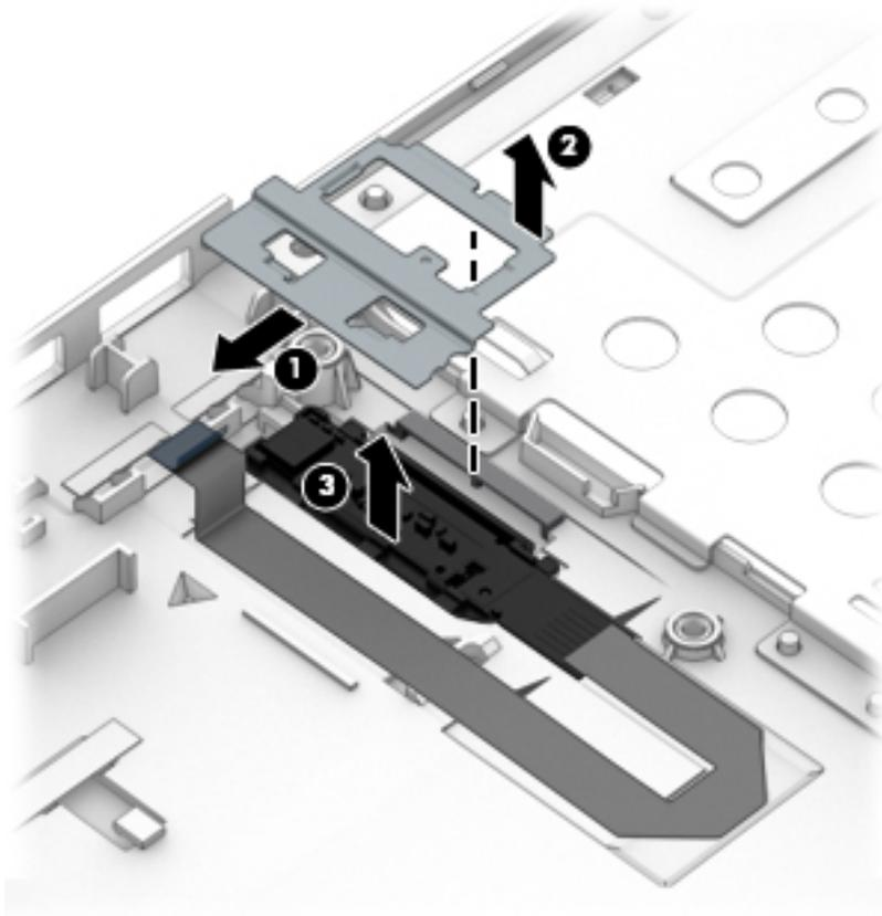
Reverse this procedure to install the fingerprint reader assembly.
