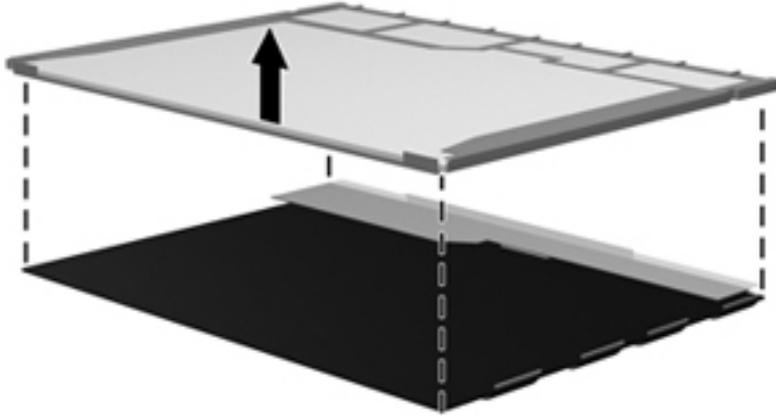
**24.** Recycle the LCD panel and backlight.
