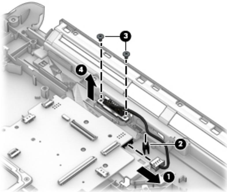
Reverse this procedure to install the battery connector cable.
