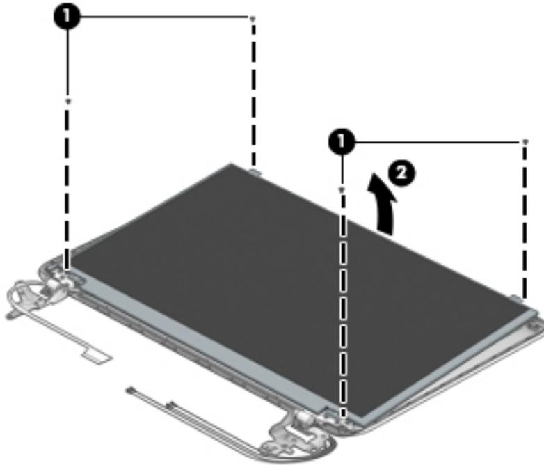
14. Rotate the display panel all the way over **(1)**, disconnect the display cable from the rear of the panel **(2)**, and then remove the display panel **(3)** from the enclosure.
