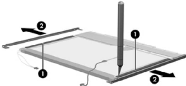
11. Remove the screws **(1)** that secure the backlight cover to the display panel.
