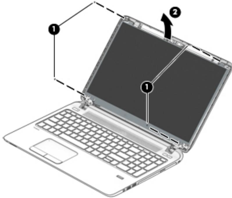
9. Rotate the display panel onto the keyboard (1), disconnect the display cable from the rear of the panel (2), and then remove the display panel (3) from the enclosure.
