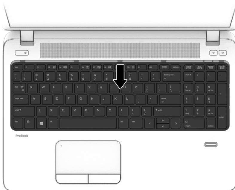
5. Rotate the top of the keyboard upward **(1)**, and then lift the keyboard up at an angle **(2)** to disengage the tabs at the bottom of the keyboard.
