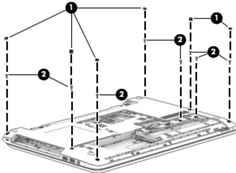
3. Remove the 11 Torx T8M2.5×3.0 screws that secure the top cover to the computer.
