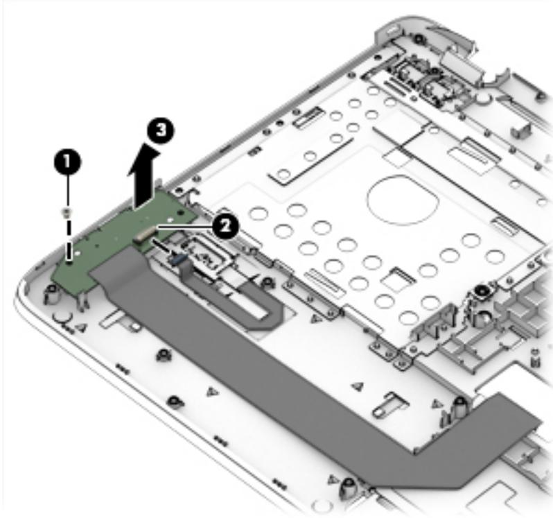
Reverse this procedure to install the USB/audio board.
