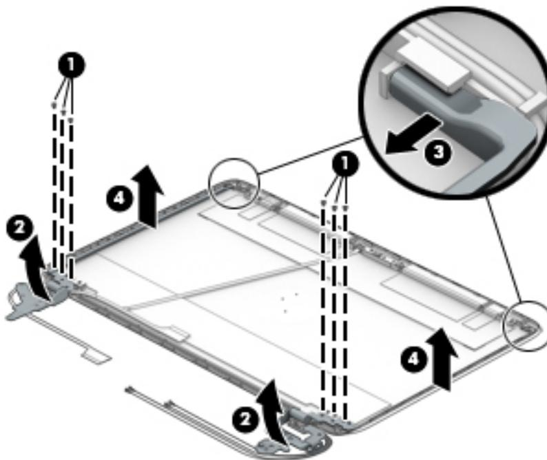
17. If it is necessary to replace the display/webcam cable, lift the display/webcam cable assembly straight up and off the display panel.
