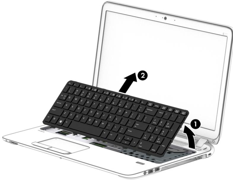
6. Rotate the keyboard until it rests on the palm rest **(1)**.
