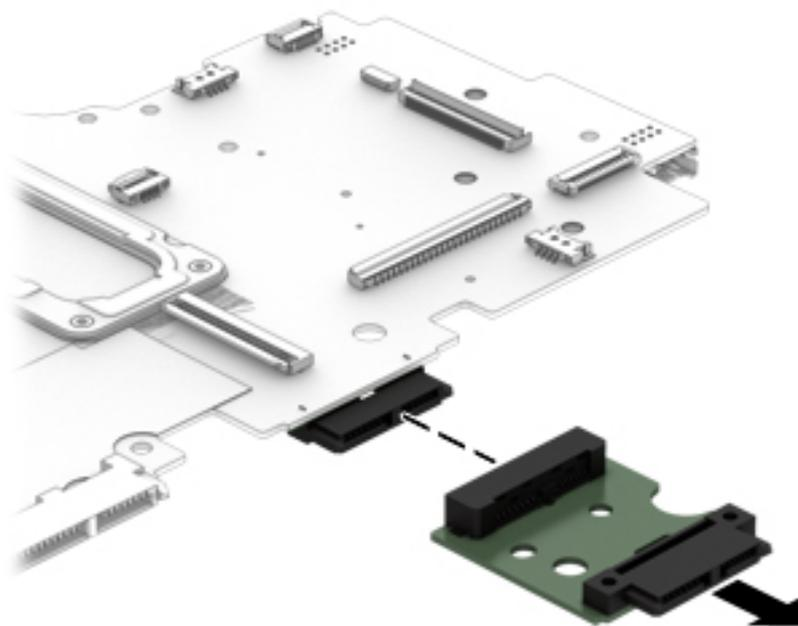
Reverse this procedure to install the optical drive extension board.
