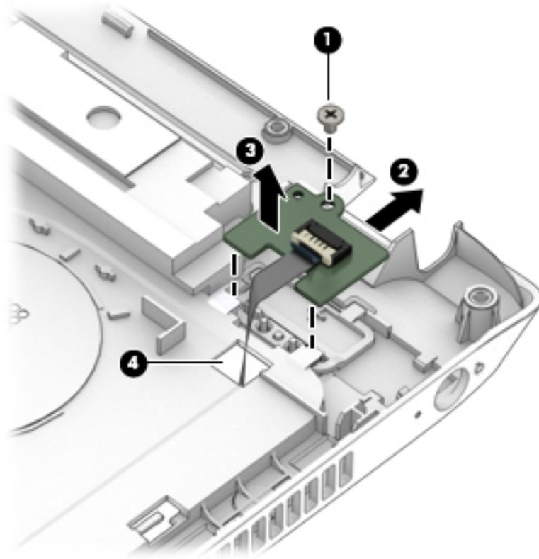
Reverse this procedure to install the power button board.
