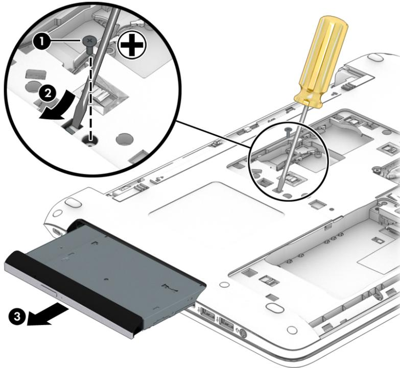
4. To remove the bracket from the optical drive, remove the Phillips PM2.0×3.0 screw **(1)** that secures the bracket to the drive, and then remove the bracket from the drive **(2)**.
