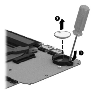
Reverse this procedure to install the RTC battery. When installing the RTC battery, make sure the "+" sign faces up.
