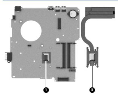
5. Reverse this procedure to install the fan/heat sink assembly. Replace the thermal material that ships with the replacement heat sink.
