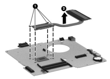
Thoroughly clean the thermal connections (1) on the system board and the heat sink (2) before replacing a heat sink onto a system board.
