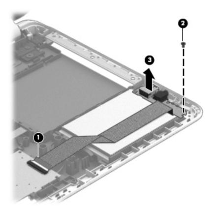
2. Lift the front of the hard drive (1) and slide the hard drive (2) forward .
