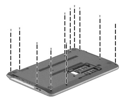
5. Remove the additional three Phillips M2.0×1.5 screws from the optical drive bay (1) and the three Phillips M2.5×6.5 screws from under the service door (2).
