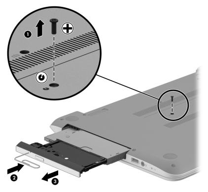
If it is necessary to replace the optical drive bracket and bezel, position the optical drive with the rear panel toward you.
