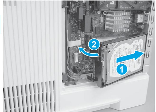
Insert the HDD cradle mounting tab in the slot in the sheet-metal (callout 1), and then rotate the connector end (callout 2) of the HDD toward the formatter.
