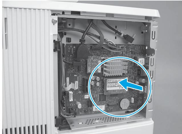
**M506 only:** Push the DIMM straight on the connector to install it. Go to step 18.
