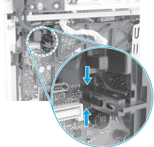
Engage the retainer with the slot in the formatter.
