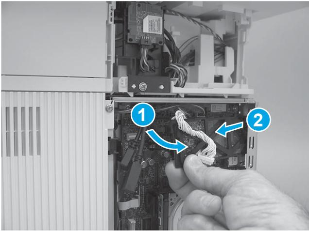
Rotate the connector end of the fax PCA out and away from the formatter (callout 1), and then slide it as shown (callout 2) to remove it.
