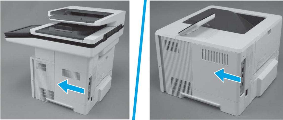
Slide the formatter cover towards the front of the printer to install it.
