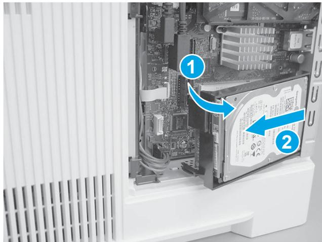
Rotate the connector end of the HDD out and away from the formatter (callout 1), and then slide it as shown (callout 2) to remove it.
