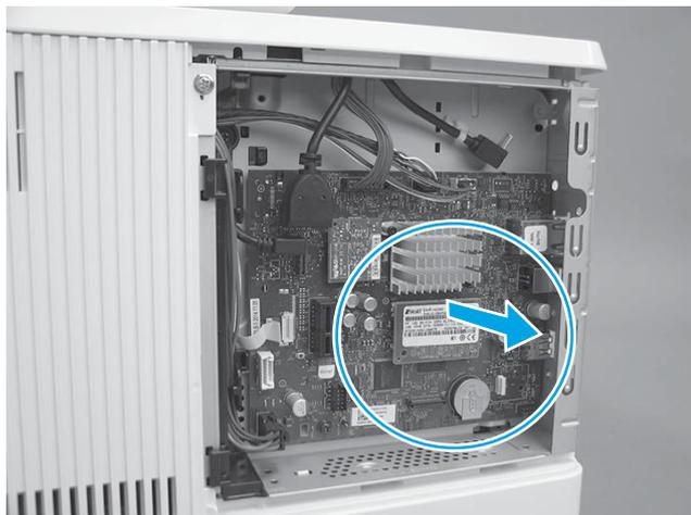
**M506 only:** Locate the DIMM component on the formatter, and then pull it straight off of the formatter to remove it.
