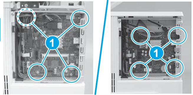
**IMPORTANT:** Take note of all empty connectors on the formatter before disconnecting any wire harnesses or flat-flexible cables (FFCs). Some empty connectors might not be visible until other items—like the hard-disk drive—are removed, so pay close attention while removing the formatter and accessories items.
