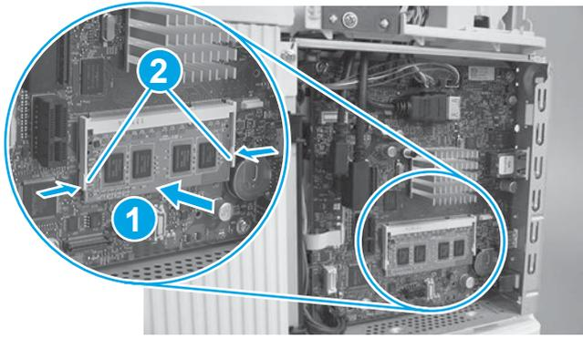
Rotate the bottom edge of the DIMM toward the holder (callout 1), and then make sure that the two locking arms snap into place (callout 2).
