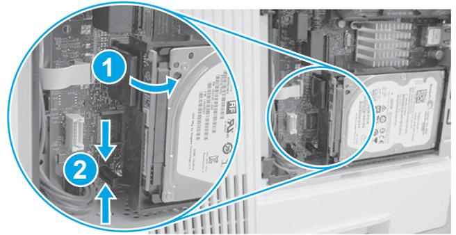
**NOTE:** Hard-disk drive (HDD) models only. For all other models, skip this step and go to **Step 9**. Release the locking connector (callout 1), and then pinch the retainer (callout 2) to release it.
