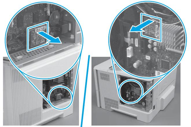
**NOTE:** M506 printers and M527dn models only. For all other models, skip this step and go to **Step 10** (M506) or **Step 11** (M527). Locate the embedded MultiMedia Card (eMMC) component on the formatter, and then pull it straight off of the formatter to remove it.
