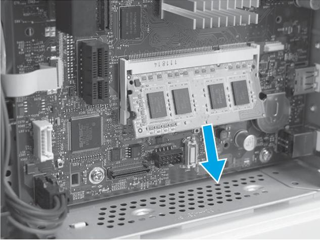
**M527 only:** Pull the DIMM down and away from the holder to remove it.
