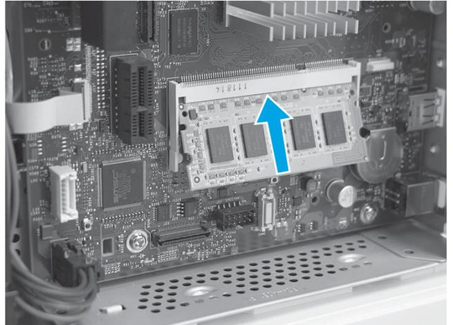
**M527 only:** Insert the top edge of the DIMM in the holder.
