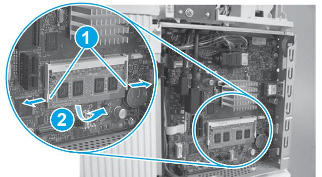
**M527 only:** Locate the DIMM component on the formatter, release two locking arms (callout 1), and then let the bottom edge of the DIMM rotate away from the holder (callout 2).
