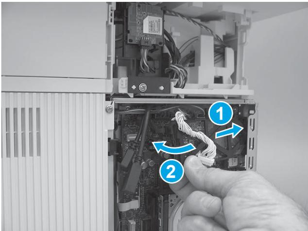
Insert the fax PCA cradle mounting tab and fax port in the slots in the sheet-metal plate (callout 1), and then rotate the connector end of the fax PCA toward the formatter (callout 2).
