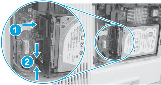
Make sure that the locking connector (callout 1) latches and that the standoff (callout 2) engages with the slot in the formatter (it might be necessary to pinch the retainer to engage it with the slot).
