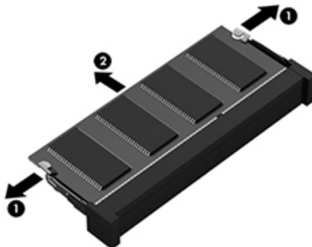
Reverse this procedure to install an expansion memory module.
