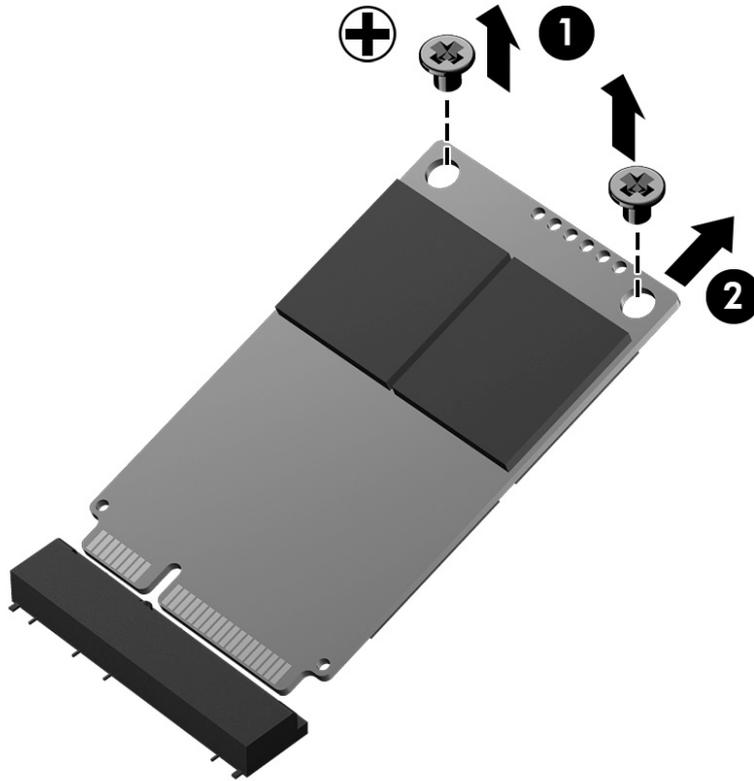
Reverse this procedure to install the solid-state drive.
