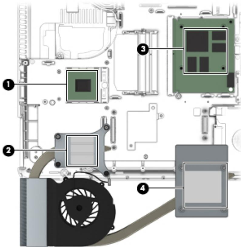
Reverse this procedure to install the graphics subsystem heat sink.
