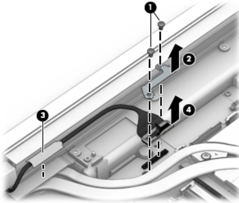
17. Remove the two Torx T8M2.5×7.0 screws (1) that secure the display assembly to the computer.
