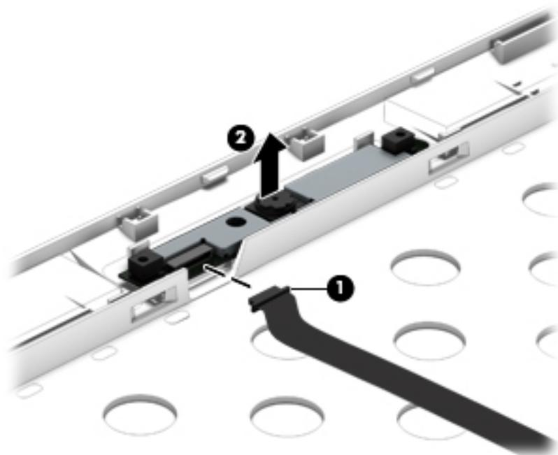
Reverse this procedure to install the webcam/microphone module.
