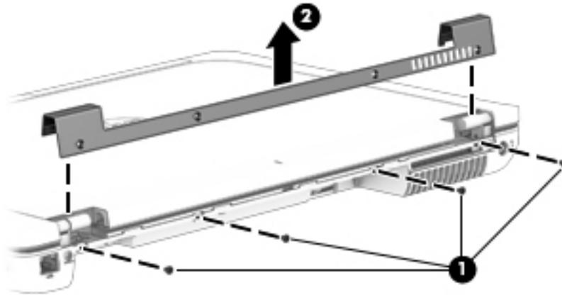
10. Remove the two Torx T8M2.5×7.0 screws that secure the display assembly to the computer.
