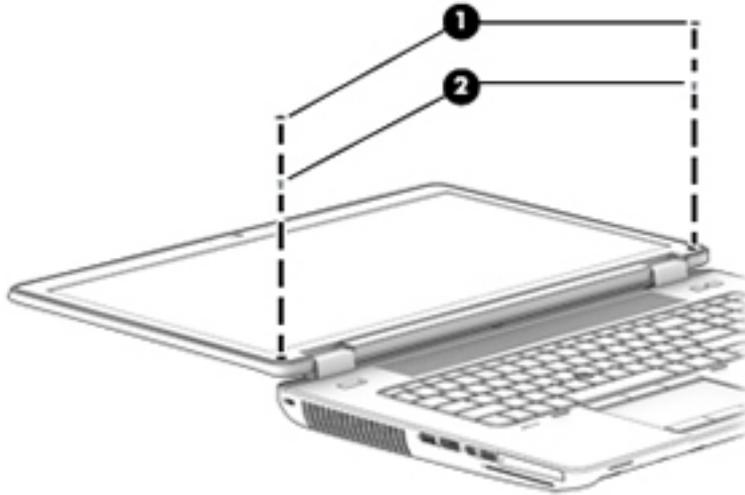
4. Flex the inside edges of the bottom edge **(1)**, the left and right sides **(2)**, and the top edge **(3)** of the display bezel until the bezel disengages from the display enclosure and then remove the bezel **(4)**.
