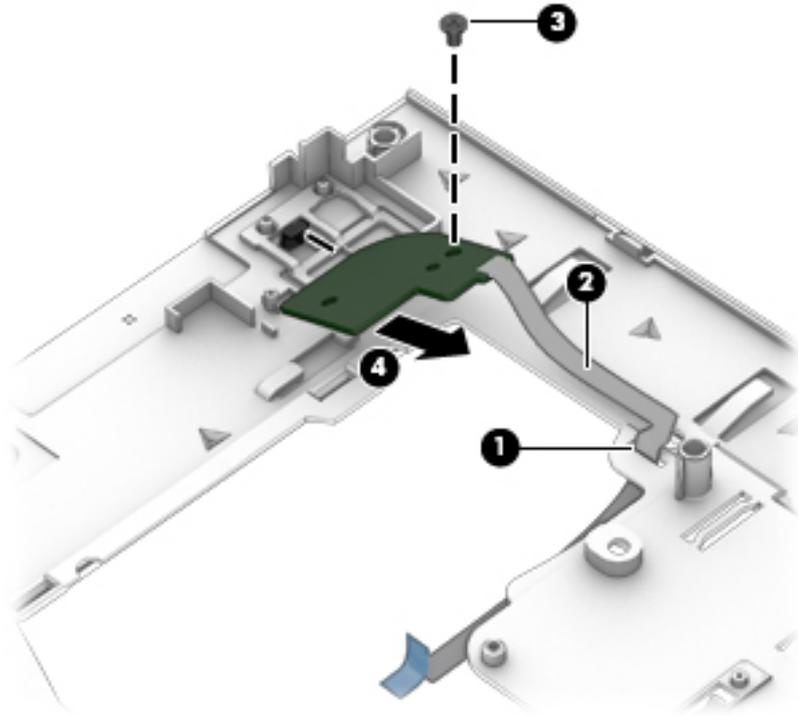
Reverse this procedure to install the power button board.
