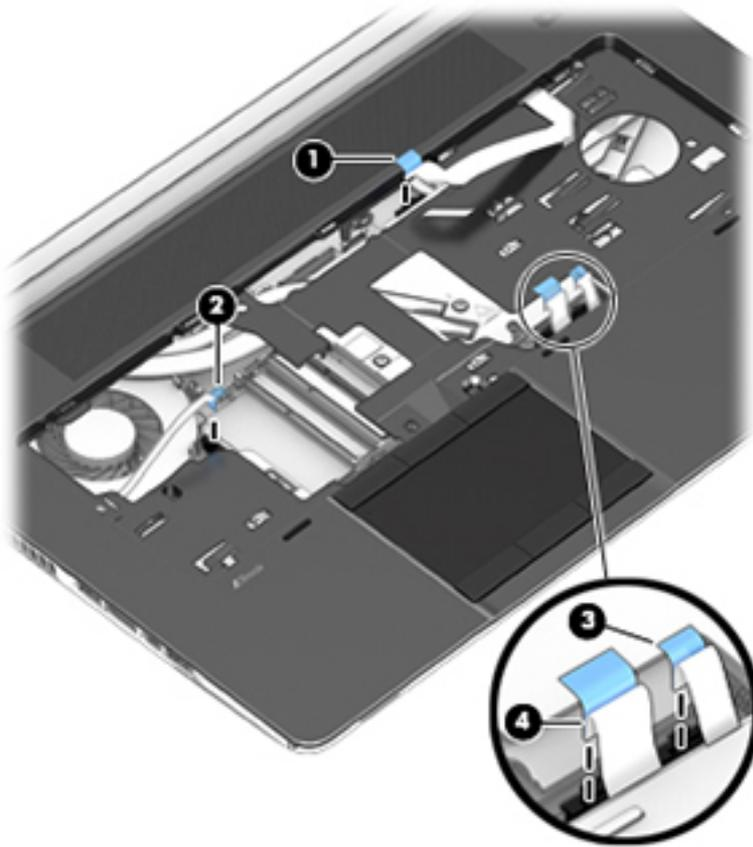
8. Starting at the top right, release the top cover from the base enclosure (1).
