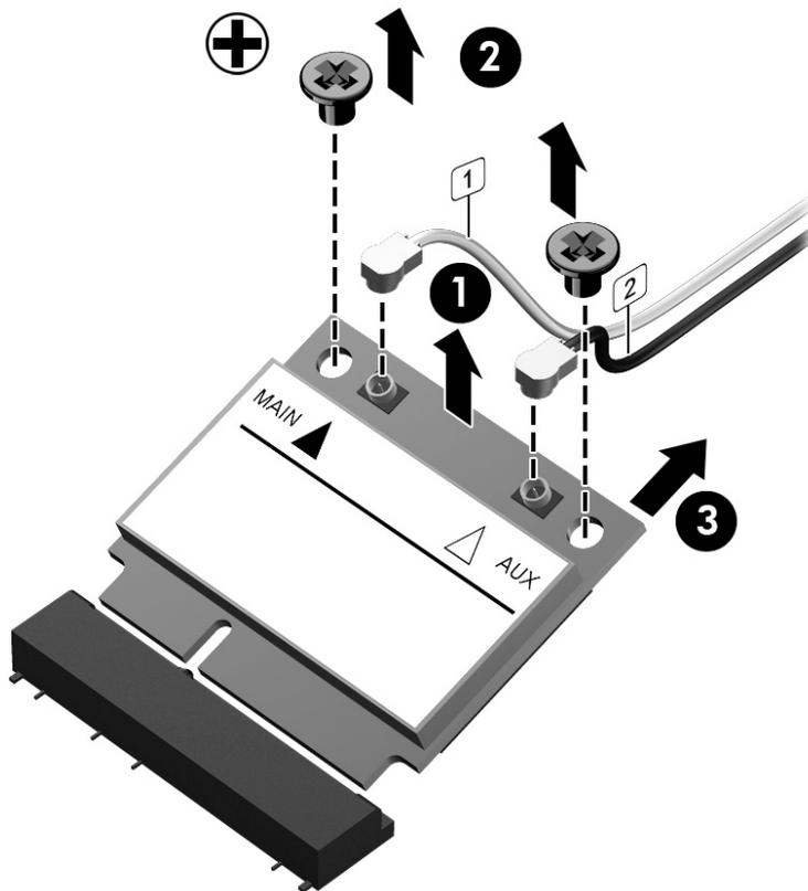
Reverse this procedure to install the WLAN module.
