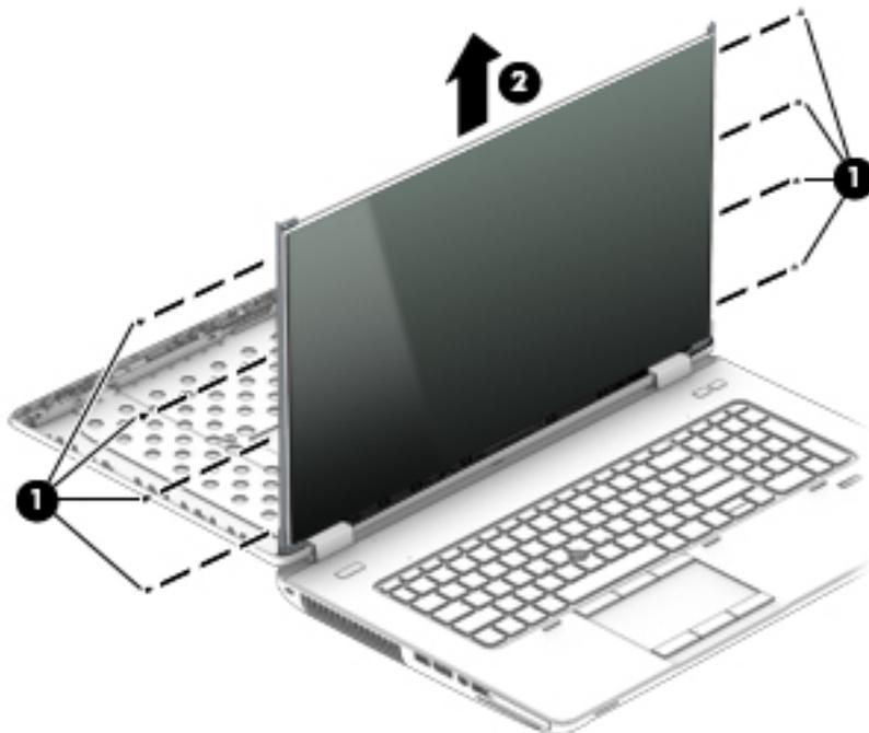
To replace the remaining display assembly components, remove the display assembly from the computer. Reverse this procedure to install the display panel. For more information, see [Display assembly on page 77](#).
