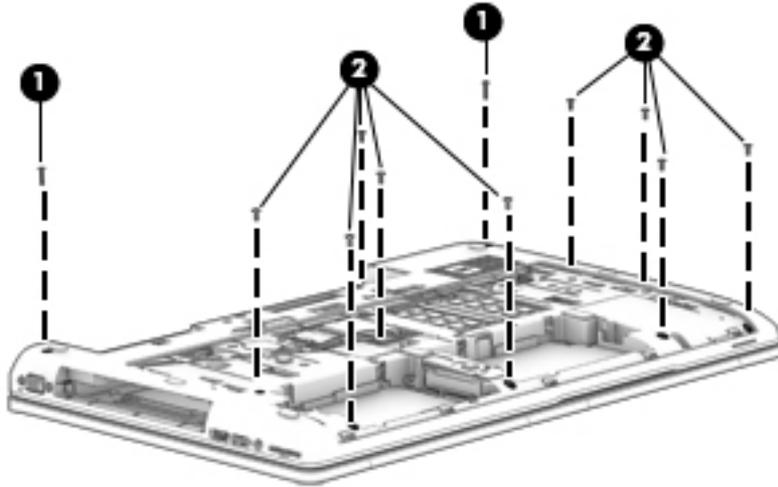
4. Remove the four Torx T8M2.5x5.0 screws inside the battery bay **(1)** and the three Torx T8M2.5x5.0 screws in the optical drive/upgrade drive bay **(2)**.
