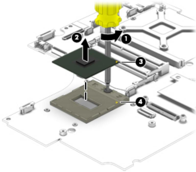
Reverse this procedure to install the processor.
