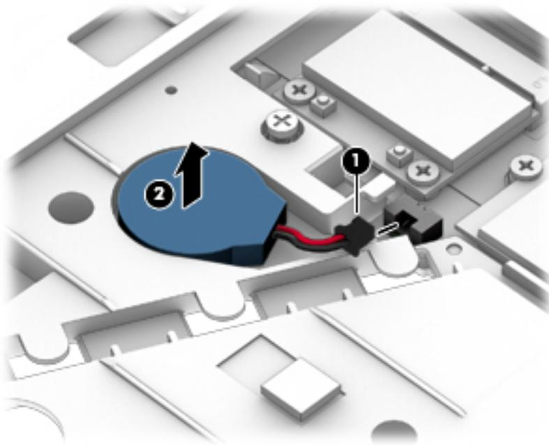
3. Remove the RTC battery.
