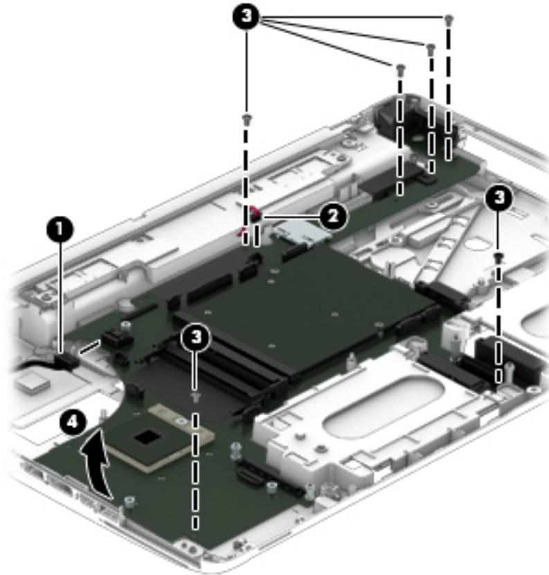
When replacing the system board, note the location of the thermal material on the system board (1) and the base enclosure (2).
