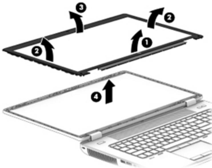
Reverse this procedure to install the display bezel.
