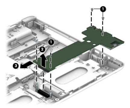
Reverse this procedure to install the audio/USB board.
