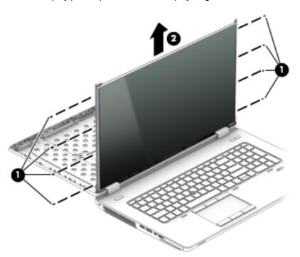
To replace the remaining display assembly components, remove the display assembly from the computer. Reverse this procedure to install the display panel. For more information, see <u>Display assembly on page 77</u>.
