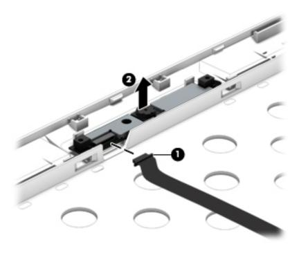
Reverse this procedure to install the webcam/microphone module.
