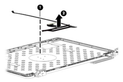
Reverse this procedure to install the display assembly.
