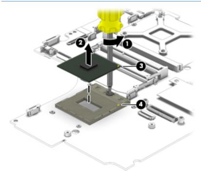
Reverse this procedure to install the processor.
