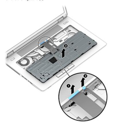
Reverse this procedure to install the keyboard.
