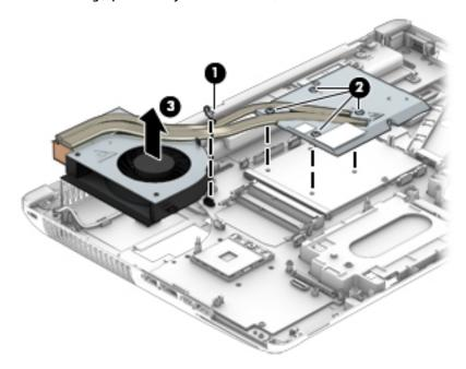
NOTE: The thermal material must be thoroughly cleaned from the surfaces of the graphics subsystem heat sink and the graphics board each time the graphics subsystem heat sink is removed. Thermal material is used on the system board component closest to the fan (1) and the heat sink component that services it (2), as well as on the graphics board (3) and various locations on the graphics subsystem heat sink section (4) that services it.
