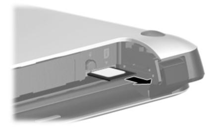
Install the SIM card by inserting it into the SIM card slot until you hear a click.
