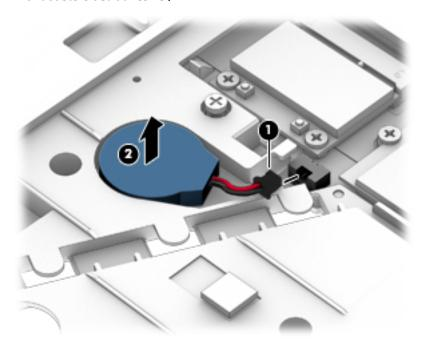
Remove the RTC battery.
