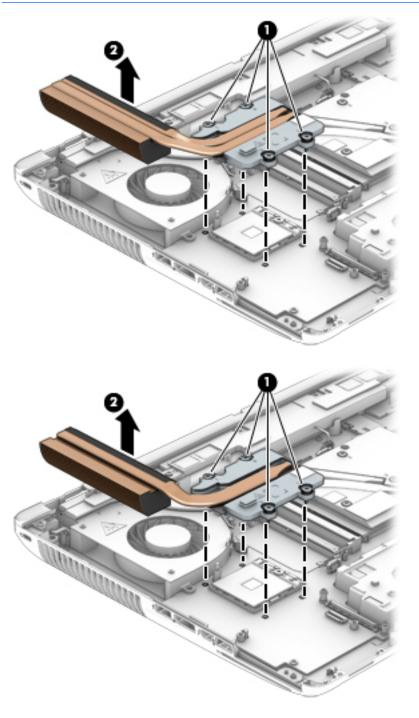
NOTE: Thermal paste located on the surfaces of the processor (1) and the processor heat sink (2). Replacement thermal paste and pads are included in the processor heat sink and processor spare part kits.
