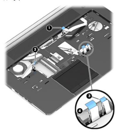
Starting at the top right, release the top cover from the base enclosure (1). 8.
