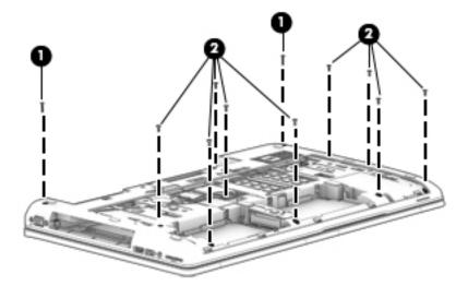
4. Remove the four Torx T8M2.5x5.0 screws inside the battery bay (1) and the three Torx T8M2.5x5.0 screws in the optical drive/upgrade drive bay (2).
