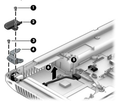
Reverse this procedure to install the power connector cable.
