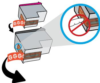
Remove plastic tape using pull tab.
