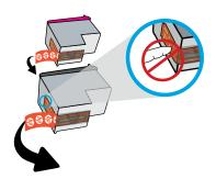
Remove plastic tape using pull tab.
