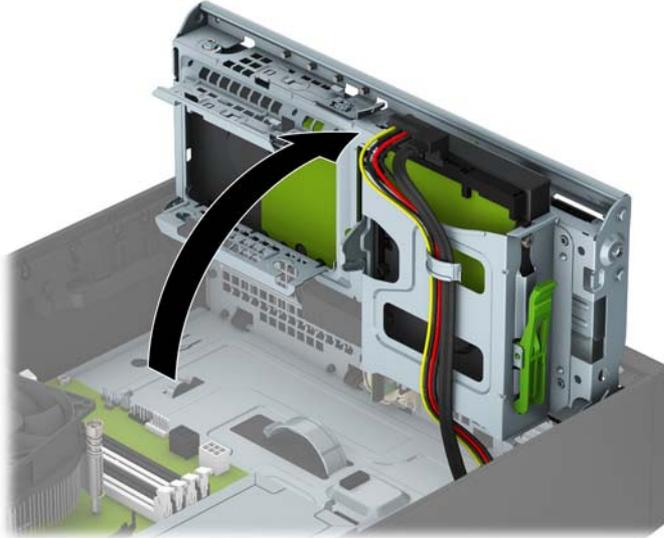
4. Disconnect the power cable (1) and data cable (2) from the rear of the hard drive. Press the latch on the side of the drive cage (3), and then slide the drive out of the drive bay (4).
