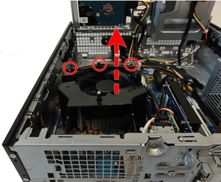
To install the fan baffle, reverse the removal procedure.
