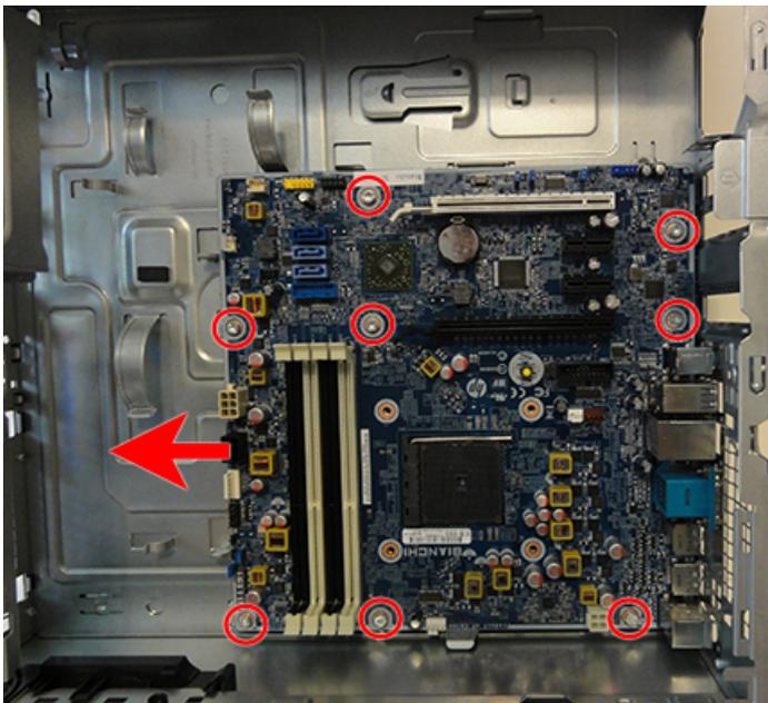
When reinstalling the system board, first insert the I/O panel back into the slots in the rear of the chassis, and then align the board with the chassis screw holes.
