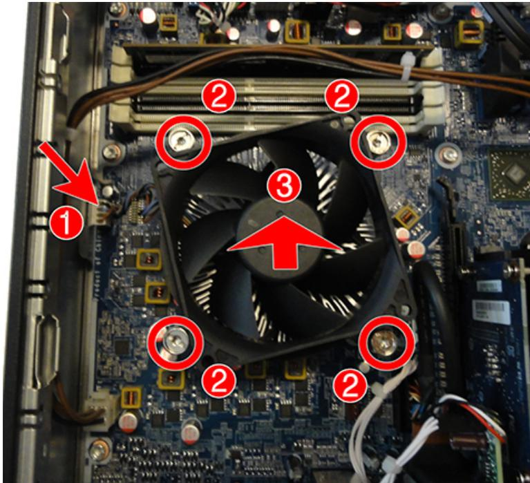
When reinstalling the fan sink, make sure that its bottom has been cleaned with an alcohol wipe and fresh thermal grease has been applied to the top of the processor.
