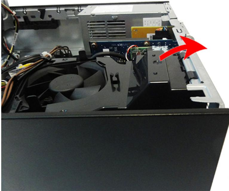
4. Pull the baffle away from the rear of the computer to disengage the clips on the baffle from the rear of the computer.
