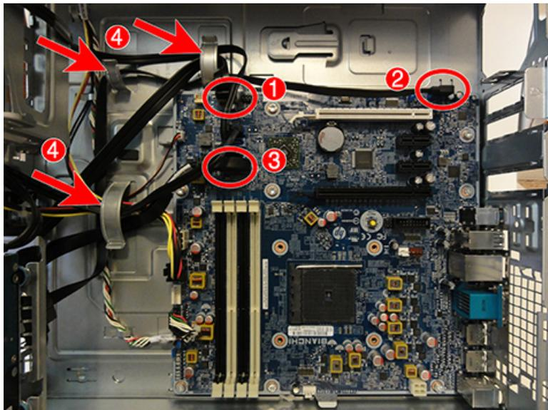
7. Remove the Torx T15 screw (1) that secures the assembly to the front of the chassis.
