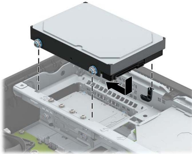
7. Connect the power cable (1) and data cable (2) to the back of the hard drive.
