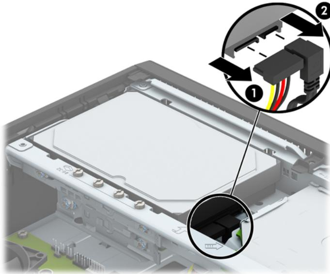
4. Pull the release lever next to the rear of the hard drive outward (1). While pulling the release lever out, slide the drive back until it stops, and then lift the drive up and out of the bay (2).
