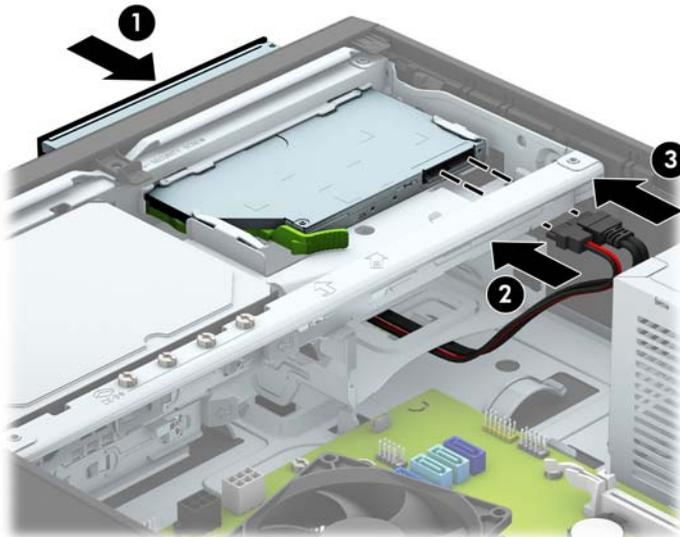
6. Connect the opposite end of the data cable to one of the light blue SATA connectors on the system board.
