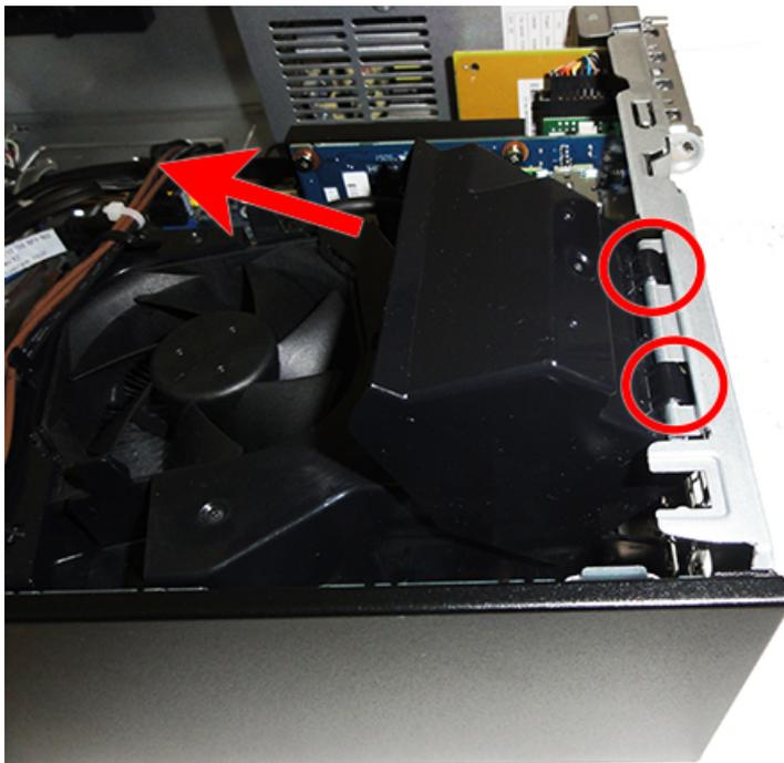
To install the small baffle, reverse the removal procedure.
