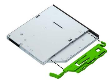
9. Slide the optical drive through the front of the chassis (1) all the way into the bay so that the green latch locks onto the chassis frame (2).
