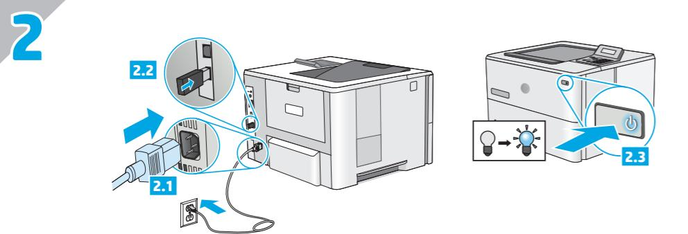
**EN** 1. **Connect the power cord between the printer and a grounded AC outlet.** Make sure the power source is adequate for the printer voltage rating. The voltage rating is on the printer label. The printer uses either 100-127 Vac or 220-240 Vac and 50/60 Hz.
