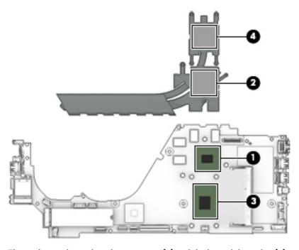
Thermal paste is used on the processor (1) and the heat sink section (2).
