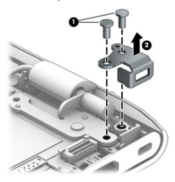
Reverse this procedure to install the security cable slot bracket.
