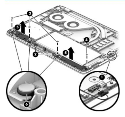
Reverse this procedure to install the front speakers.
