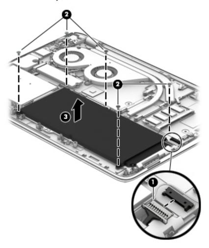
Reverse this procedure to install the battery.
