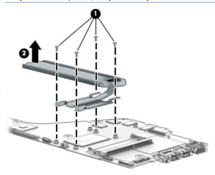
5. The thermal material must be thoroughly cleaned from the surfaces of the heat sink and the system board each time the heat sink is removed. Replacement thermal material is included with the heat sink and system board spare part kits.
