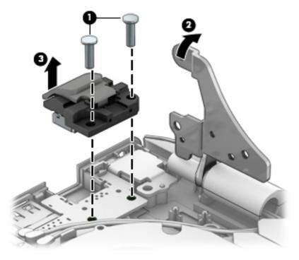
Reverse this procedure to install the RJ45 cover.
