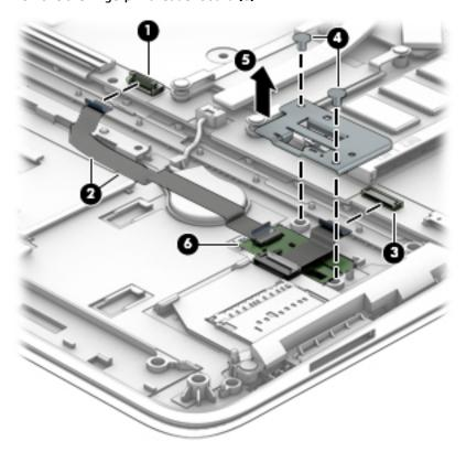
If it is necessary to replace the fingerprint reader board cable, release the ZIF connector (1) to which the fingerprint reader board cable is attached, and then disconnect the fingerprint reader board cable (2) from the fingerprint reader board.
