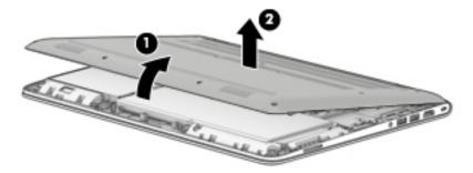
Reverse this procedure to install the bottom cover.
