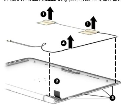
Reverse this procedure to install the display assembly subcomponents.
