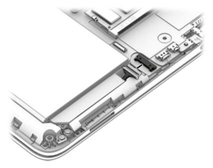
2. Remove the two Phillips PM2.5×8.8 screws (1) that secure the security cable slot bracket to the top cover.
