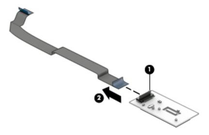
Reverse this procedure to install the fingerprint reader board.
