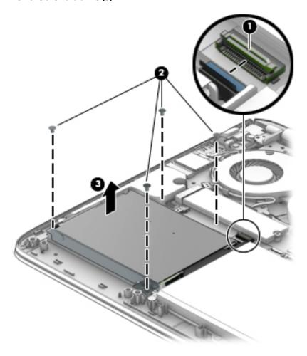
If it is necessary to disassemble the hard drive:
