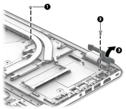
6. Lift the left side of the system board (1) until it rests at an angle.
