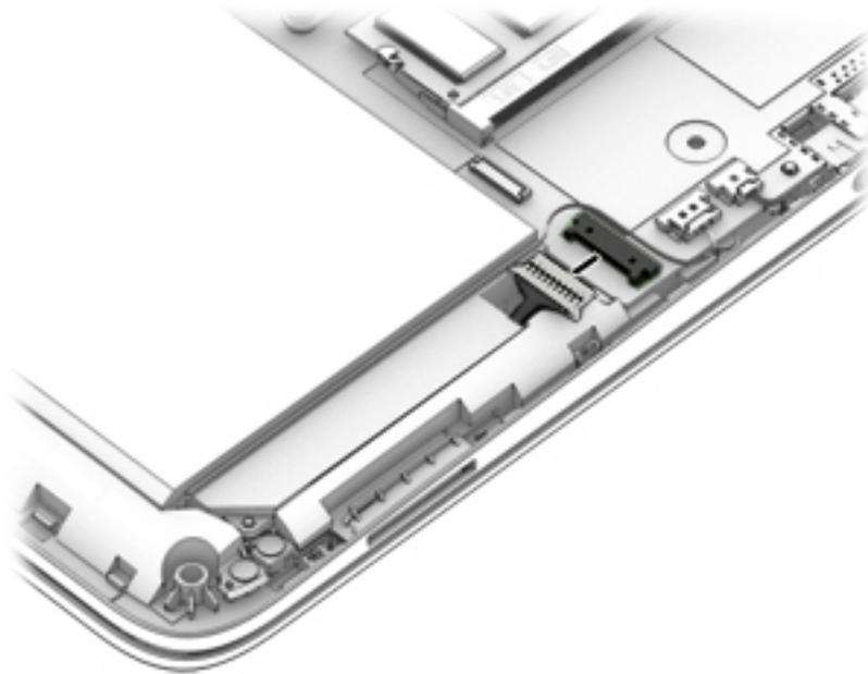
2. Disconnect the subwoofer cable **(1)** from the system board.
