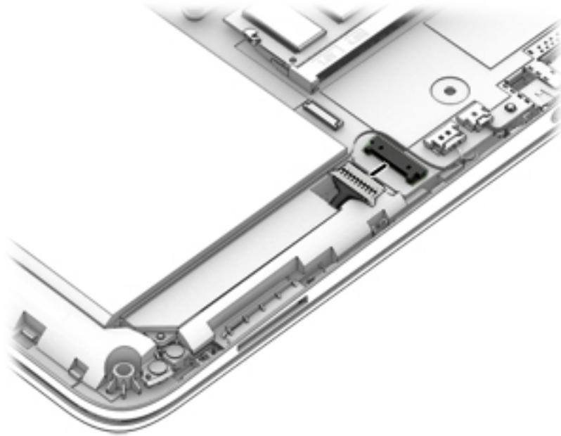
2. Remove the two Phillips PM2.5×8.8 screws **(1)** that secure the RJ45 cover and the right display hinge to the top cover.
