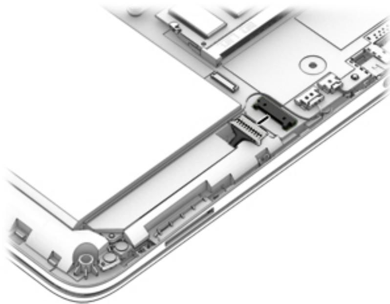
2. Release the zero insertion force (ZIF) connector **(1)** to which the hard drive cable is connected, and then disconnect the hard drive cable from the system board.
