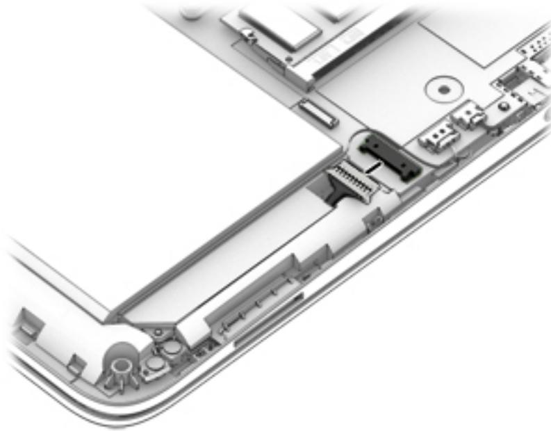
2. Disconnect the WLAN antenna cables **(1)** from the WLAN module terminals.
