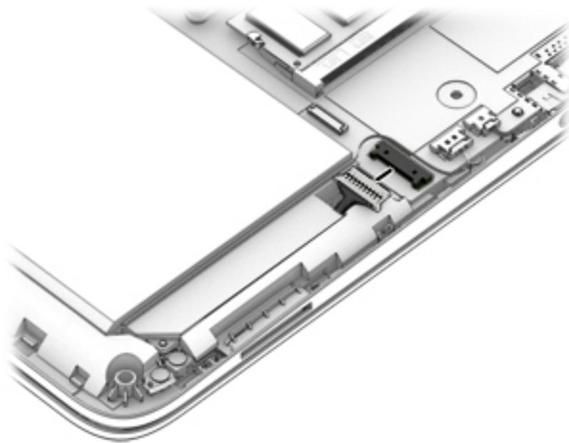
2. Release the ZIF connector **(1)** to which the fingerprint reader board cable is attached, and then disconnect the fingerprint reader board cable from the fingerprint reader board.
