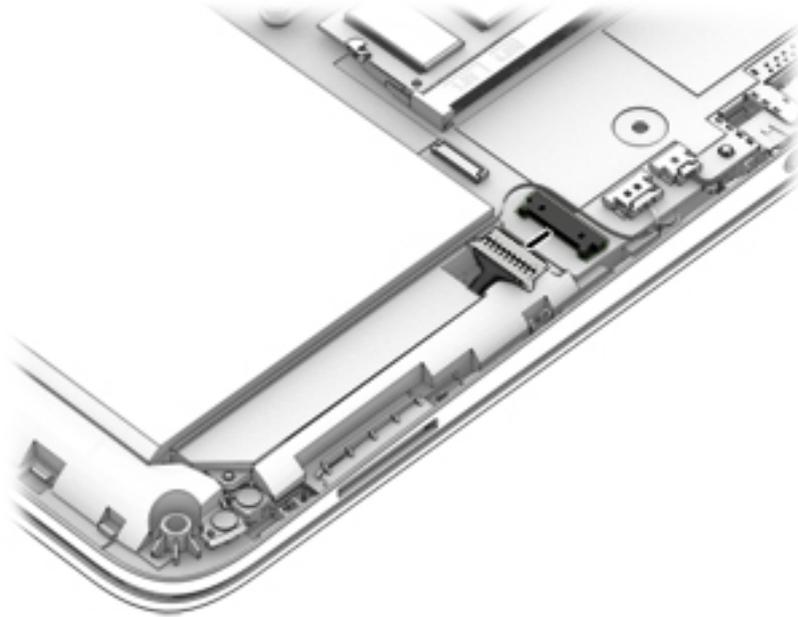
2. Release the fingerprint reader board cable **(1)** from the TouchPad board. (The fingerprint reader board cable is secured to the TouchPad board with double-sided adhesive.)
