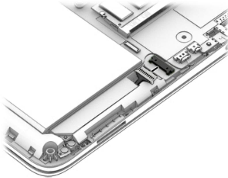
2. Disconnect the front speakers cable **(1)** from the system board.
