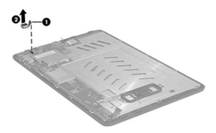
Reverse this procedure to install the rear-facing webcamera.
