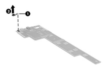
Reverse this procedure to install the front-facing webcamera.
