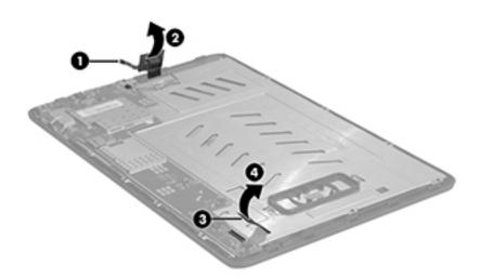
2. Disconnect the display cable (3) from the middle frame (4).
