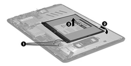
Reverse this procedure to install the battery.
