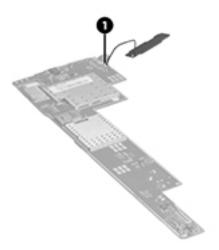
Reverse this procedure to install the antenna board.
