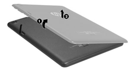
Reverse this procedure to install the back cover.
