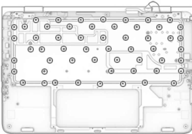
2. Remove the keyboard shields **(1)**.
