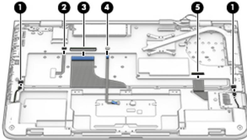
10. Remove the Phillips PM2.0×2.6 broad head screw (1) and the Phillips PM2.0×2.7 screw (2) that secure the system board to the top cover.
