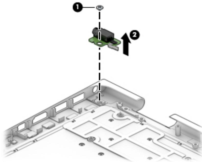
Reverse this procedure to install the audio jack board.
