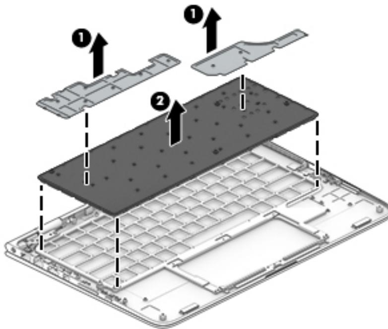
Reverse this procedure to install the keyboard.
