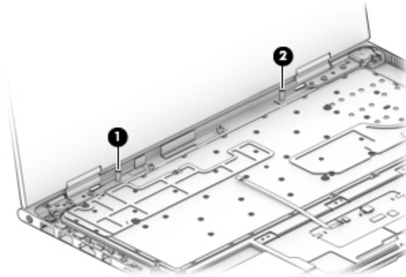
4. Remove the four Phillips PM2.5×4.1 screws **(1)** that secure the display assembly to the top cover.
