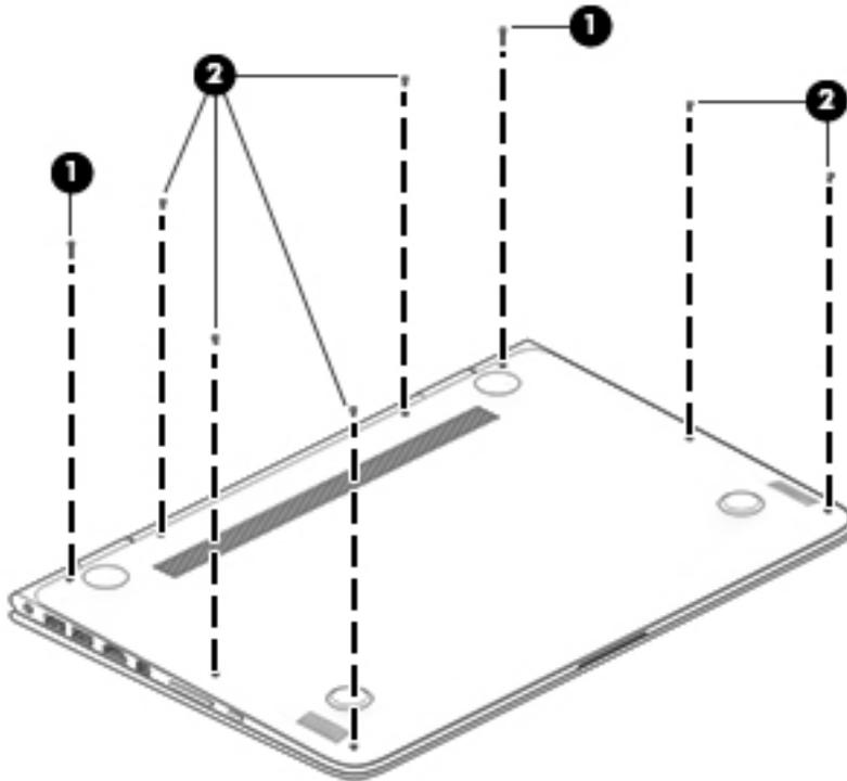
4. Separate the rear edge of the bottom cover **(1)** from the top cover until it rests at an angle.
