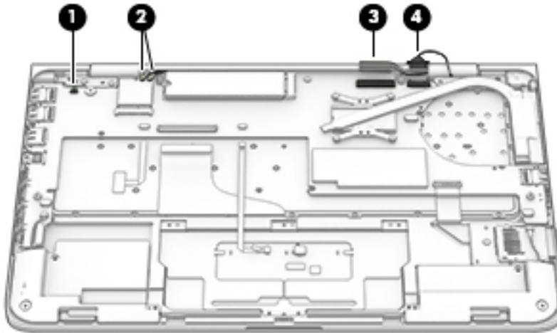
5. Disconnect the speaker cables **(1)** from the system board.
