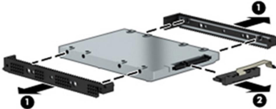
Reverse this procedure to reassemble and install the hard drive.
