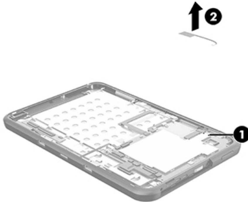
15. Remove the WLAN auxiliary antenna cable and transceiver.
