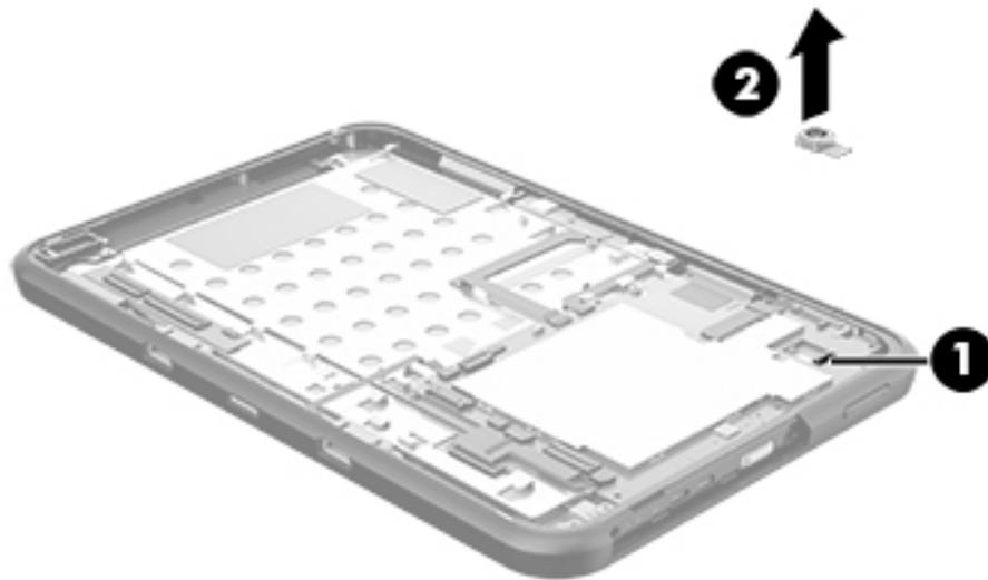
3. Remove the rear-facing webcam and cable.
