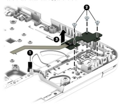
Reverse this procedure to install the function button board.
