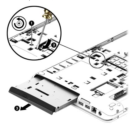
Reverse this procedure to install the optical drive.
