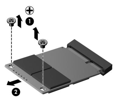
Reverse this procedure to install the solid-state drive.
