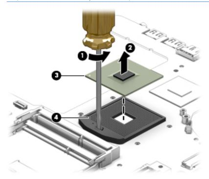
Reverse this procedure to install the processor.
