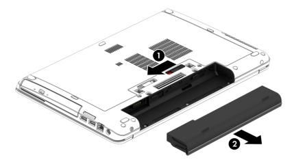
Reverse this procedure to install the battery.
