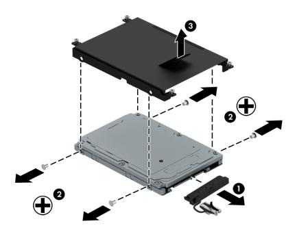
Reverse this procedure to install a hard drive.
