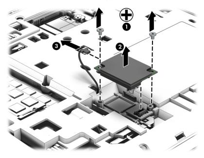
Remove the modem module.
