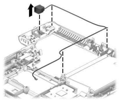
Remove the power connector cable.
