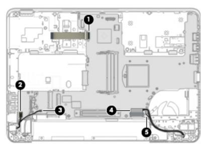
2. Remove the five Torx screws (1) and the Phillips screw (2) that secure the system board to the base enclosure.
