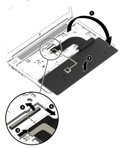
Reverse this procedure to install the keyboard.
