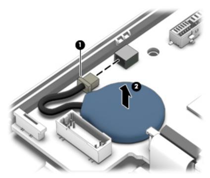
Remove the RTC battery and cable.
