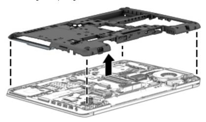
Reverse this procedure to install the base enclosure.
