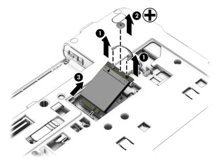
NOTE: If the WWAN antenna cables are not connected to the terminals on the WWAN module, protective sleeves should be installed on the antenna connectors, as shown in the following illustration.
