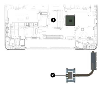
Thermal locations for computer models equipped with discrete graphics are shown in the following illustration:
