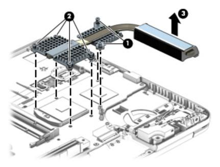
NOTE: The thermal material must be thoroughly cleaned from the surfaces of the fan/heat sink assembly and the system board components each time the fan and heat sink assembly is removed. Replacement thermal material is included with the fan/heat sink assembly, processor, and system board spare part kits.
