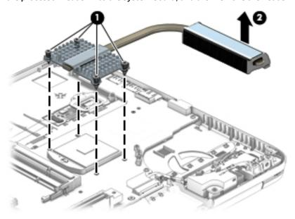
• For computer models equipped with discrete graphics, following the 1, 2 sequence stamped into the graphics board heat sink, loosen captive screws (1). Following the 1 through 4 sequence stamped into the processor heat sink, loosen the four Phillips captive screws that secure the processor heat sink to the system board (2). Then, remove the heat sink assembly (3).
