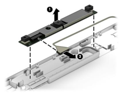
Remove the webcamera/microphone module. c.
