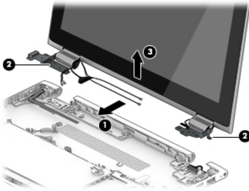
5. If it is necessary to replace the display panel assembly or any of the display assembly internal components:
