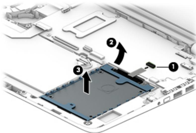
4. If it is necessary to replace the hard drive connector adapter, slide the adapter **(1)** off of the front end of the hard drive.
