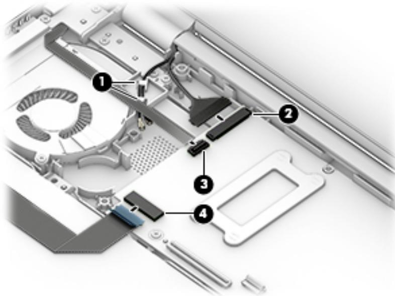
3. Disconnect the following cables from the system board:
