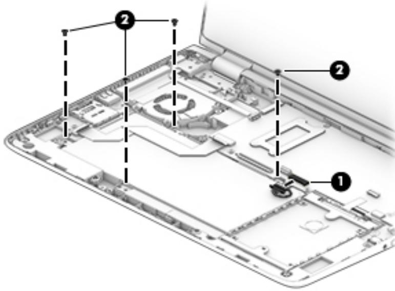
3. Detach the connector board cable **(1)** from the battery. (The connector board cable is attached to the battery with double-sided adhesive.)
