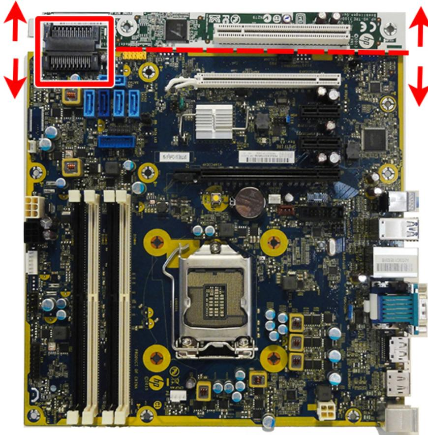
When reinstalling the system board, first insert the I/O panel back into the slots in the rear of the chassis, and then align the board with the chassis screw holes.
