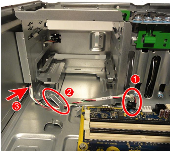
6. From the front of the chassis, press the tab on the top of the power switch **(1)**, and then rotate the top to of the assembly downward and pull the assembly out of the front of the chassis **(2)** while threading the cables through the hole in the front of the chassis.
