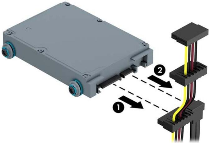
4. Remove the drive by pulling the release tab away from the drive (1) and sliding the drive out of the bay (2).
