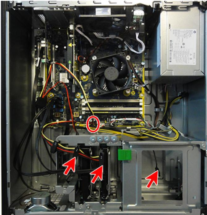
To reinstall the drive power cable, reverse the removal procedure.
