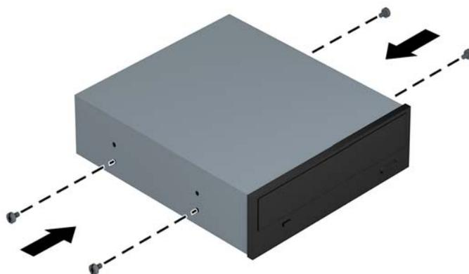
5. Slide the drive into the drive bay, making sure to align the mounting screws with the mounting slots, until the drive snaps into place.
