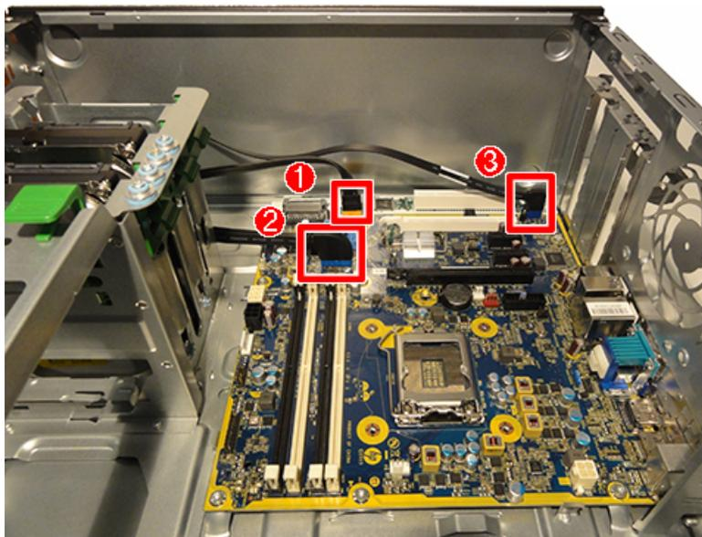
5. Remove the Torx T15 screw **(1)** that secures the assembly to the chassis, pull the right side of the assembly **(2)** to disengage it from the chassis, and pull the assembly out of the front of the chassis **(3)** while threading the cables through the hole in the front of the chassis.
