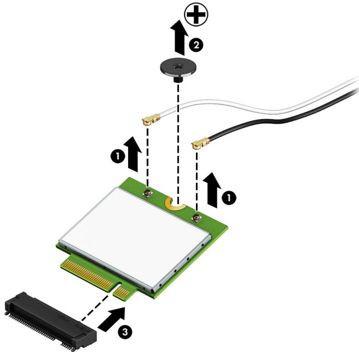
Reverse this procedure to install the WLAN module.
