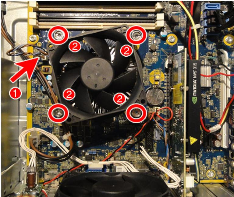
When reinstalling the fan sink, make sure that its bottom has been cleaned with an alcohol wipe and fresh thermal grease has been applied to the top of the processor.
