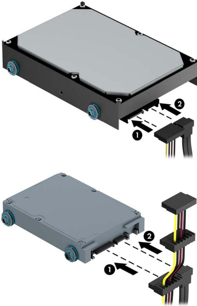
6. If installing a new drive, connect the opposite end of the data cable to the appropriate system board connector.
