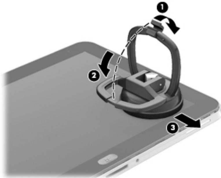
17. Slide the display assembly **(1)** to the left until the display assembly cables and connectors are accessible.
