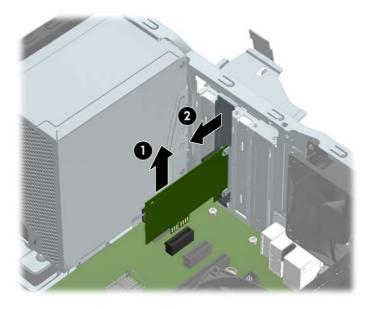
c. If you are removing a PCI Express x16 card, pull the retention arm on the back of the expansion socket away from the card and carefully rock the card back and forth until the connectors pull free from the socket. Lift the card straight up then away from the inside of the chassis to remove it. Be sure not to scrape the card against other components.
