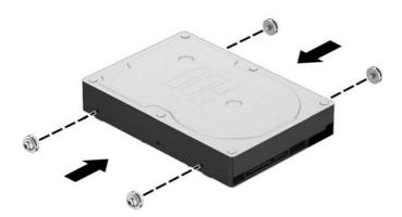
8. Slide the drive into the drive bay, making sure to align the mounting screws with the guide slots, until the drive snaps into place.
