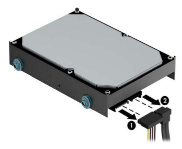
7. Pull the green latch next to the drive outward (1) and slide the drive out of the bay (2).
