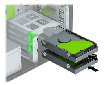
9. Connect the power cable (1) and data cable (2) to the rear of the hard drive.
