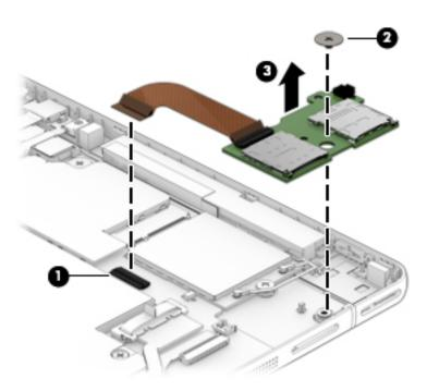
Reverse this procedure to install the card reader board.
