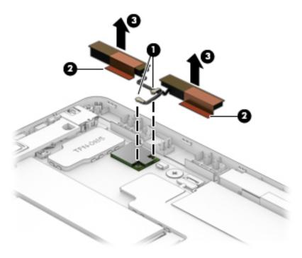
Reverse this procedure to install the WLAN antenna.
