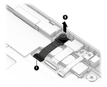
3. Remove the front-facing webcam and cable.
