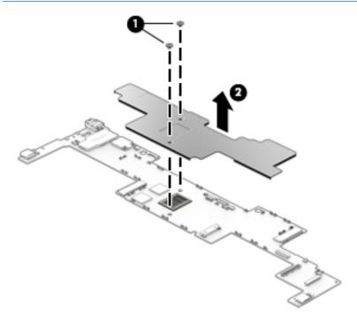
NOTE: The thermal material must be thoroughly cleaned from the surfaces of the heat sink and the system board each time the heat sink is removed. Replacement thermal material is included with the heat sink and system board spare part kits. Thermal paste is used on the system board (1) and the section of the heat sink (2) that services it.
