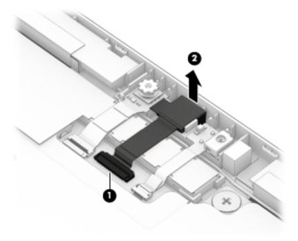
3. Remove the rear-facing webcam and cable.
