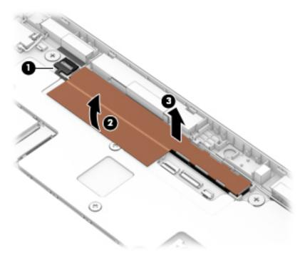
4. Remove the 3D camera board and cable.
