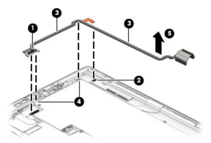
Reverse this procedure to install the display panel cable.
