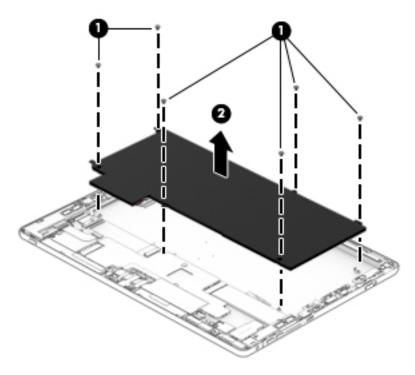
Reverse this procedure to install the battery.
