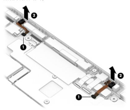
Remove the microphones and cables.
