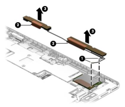
Reverse this procedure to install the WWAN antenna.
