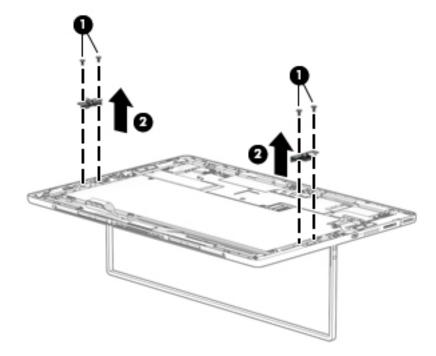
Reverse this procedure to install the kickstand retention assemblies.
