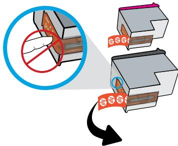
Remove plastic tape using pull tab.
