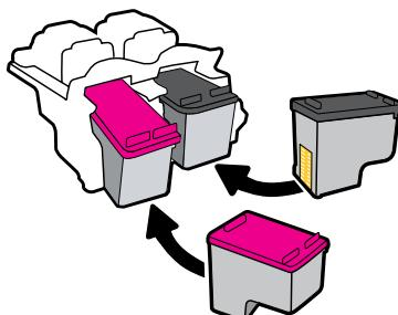
Insert cartridges into slots.
