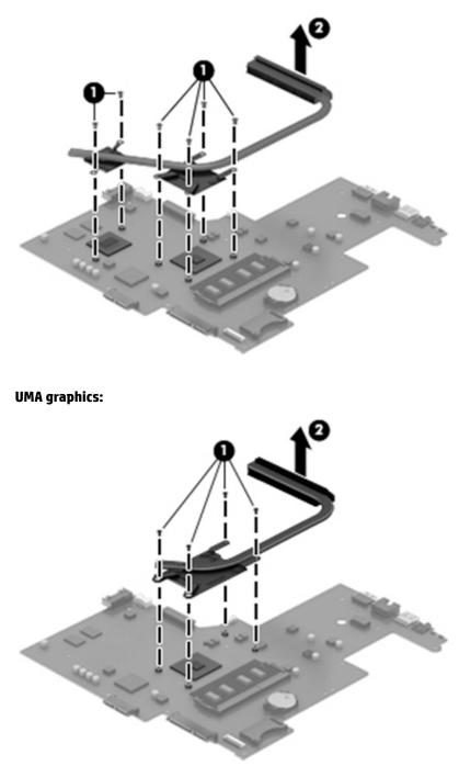
• **Discrete graphics:** Thermal paste is used on the processor and associated heat sink area (1)(2), as well as the graphics chip and associated heat sink area (3)(4).
