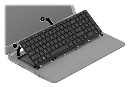
5. Rotate the keyboard over onto the palm rest (1), and the lift the ZIF connector (2) and disconnect the keyboard cable from the system board (3).
