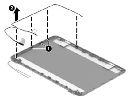
If replacing the display enclosure, be sure that the subcomponents (including the webcam/microphone module, the antenna receivers, and all associated cables and hardware) are transferred to the new enclosure.
