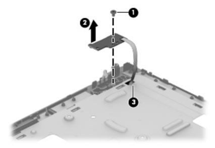
Reverse this procedure to install the power button board and cable.
