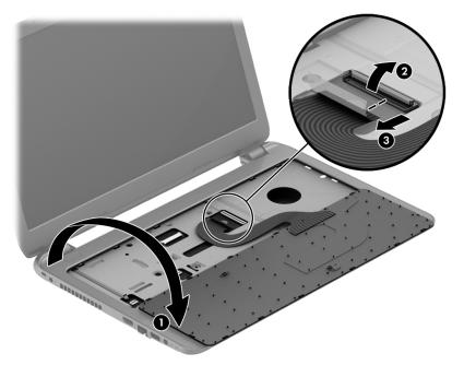
Reverse this procedure to install the keyboard.
