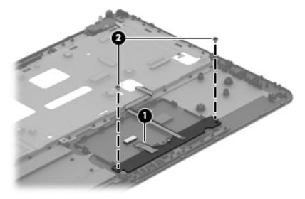
4. Remove the TouchPad button board and cable.
