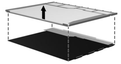
**24.** Recycle the LCD panel and backlight.
