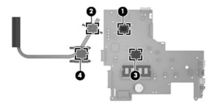
• UMA graphics: Thermal paste is used on the heat sink (1) and the processor (2).
