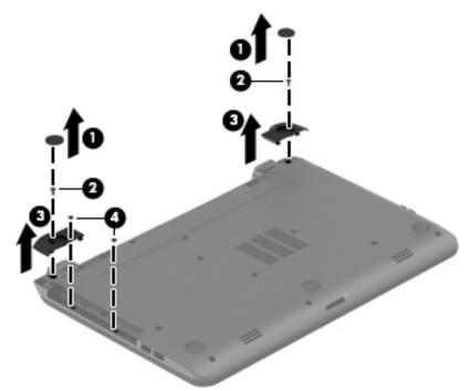
4. Remove the seven Phillips PM2.5×5.0 screws that secure the top cover to the computer.
