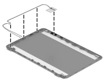
6. To remove the display/webcam cable, remove the cable from the clips built into the display enclosure (1), and then remove the cable from the display enclosure (2).
