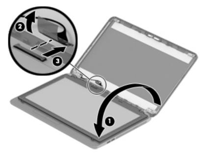
Reverse this procedure to reassemble and install the display bezel, webcam/microphone module, and display panel.
