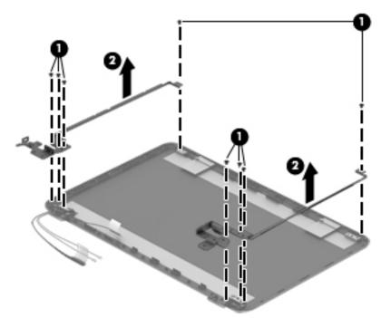
5. To remove the wireless antenna cables and transceivers, release the wireless antenna cables from the clips built into the display enclosure.
