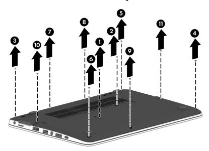
3. Remove the SD card blank and the 1 PM2.0×7.0 screw beneath it (3) that secures the bottom cover to the computer.
