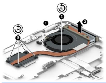
NOTE: The thermal material must be thoroughly cleaned from the surfaces of the heat sink and the system board components each time the heat sink is removed. Replacement thermal material is included with the heat sink, processor, and system board spare part kits.
