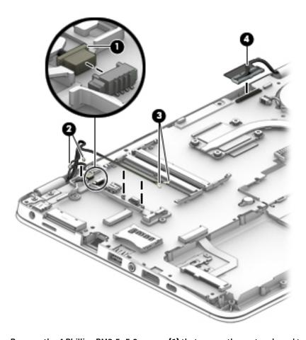
2. Remove the 4 Phillips PM2.5×5.0 screws (1) that secure the system board to the computer.
