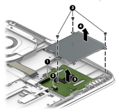
Reverse this procedure to install the card reader board.
