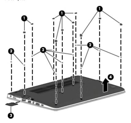
**4.** Pry up on the top (near the display hinge) of the bottom cover to disengage it from the computer **(4)**. Reverse the removal procedures to install the bottom cover.
