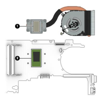
Reverse this procedure to install the heat sink/fan assembly.
