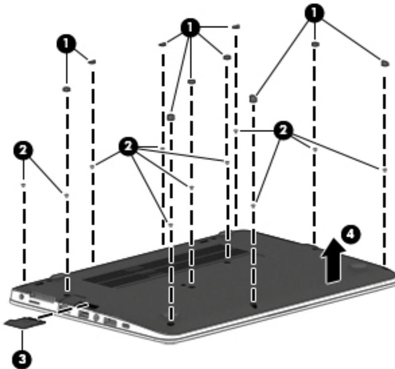
4. Pry up on the top (near the display hinge) of the bottom cover to disengage it from the computer **(4)**.
