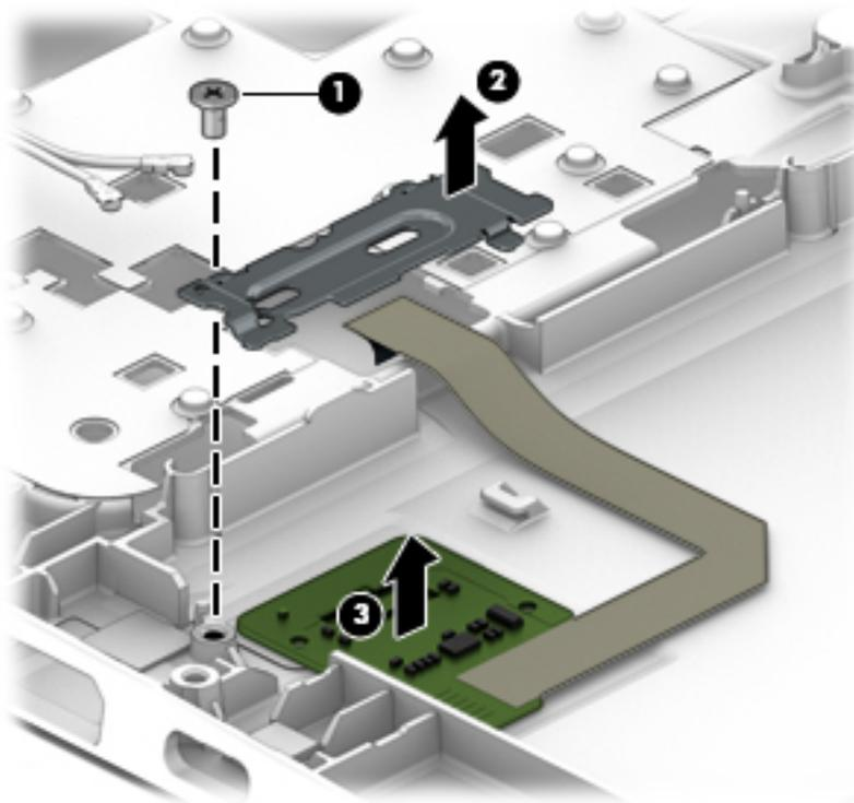
Reverse this procedure to install the fingerprint reader assembly.
