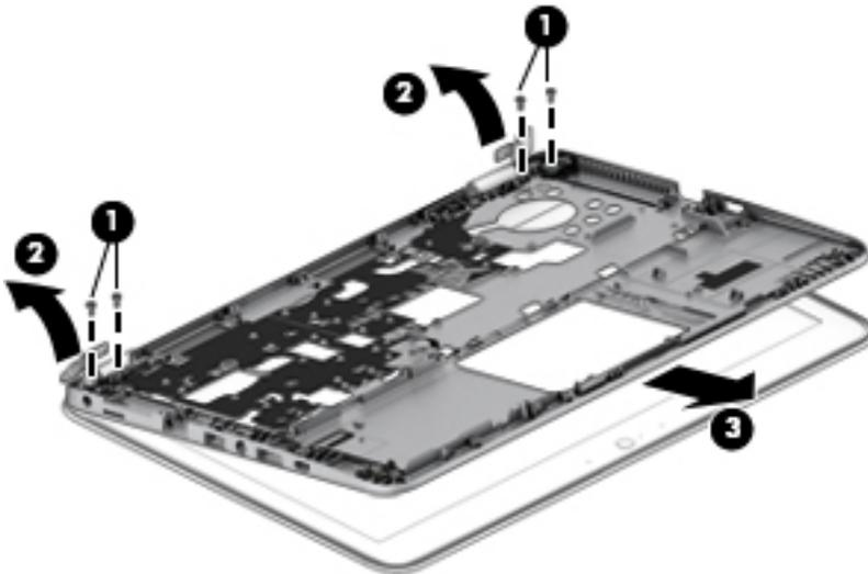
5. Lift the hinges (2) up and remove the top cover from the display assembly (3).
