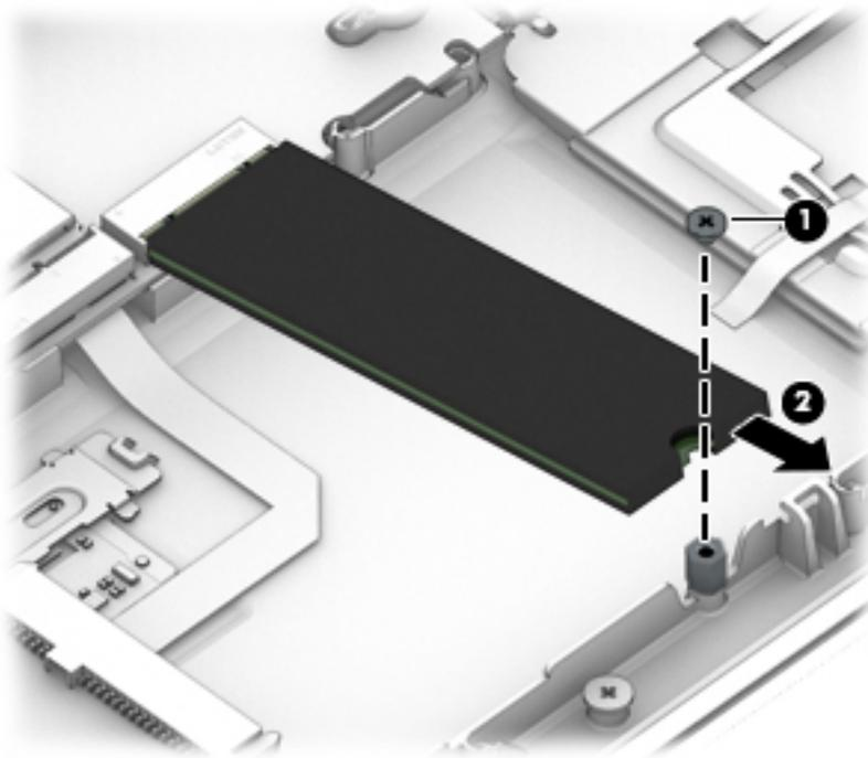
2. Remove the drive **(2)** by pulling it away from the connector.
