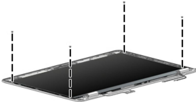
10. Rotate the display panel all the way over (1), disconnect the display cable from the rear of the panel (2), and then remove the display panel from the enclosure.
