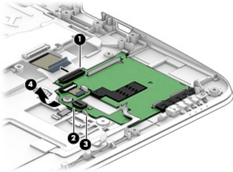
Reverse this procedure to install the card reader board.
