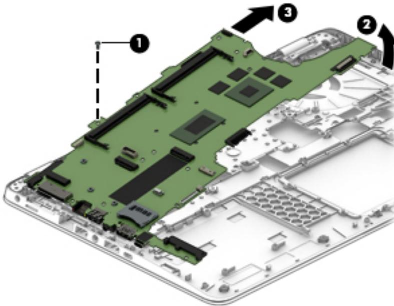
3. Lift the right side of the system board up at an angle (2).
