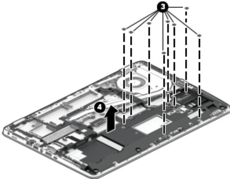
Reverse this procedure to install the internal base plate.
