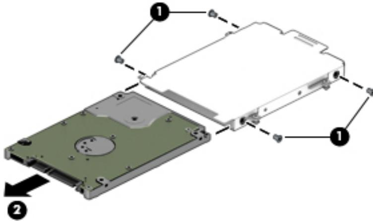
Reverse this procedure to install a hard drive.
