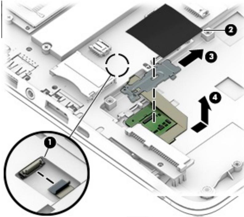
Reverse this procedure to install the fingerprint reader assembly.
