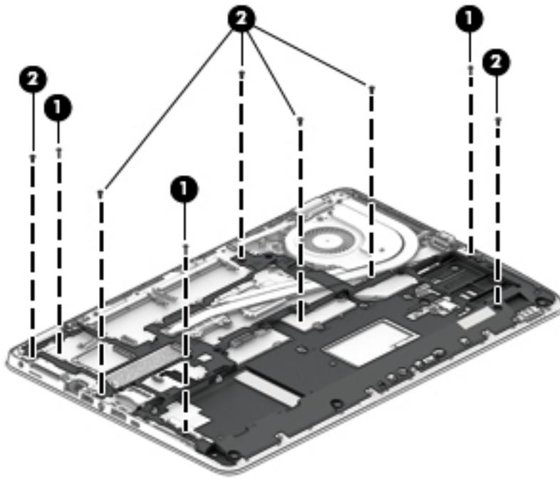
2. On 14" computers, remove 9 Phillips PM2.5x5.0 screws **(1)**, and then remove the base plate from the computer **(2)**.
