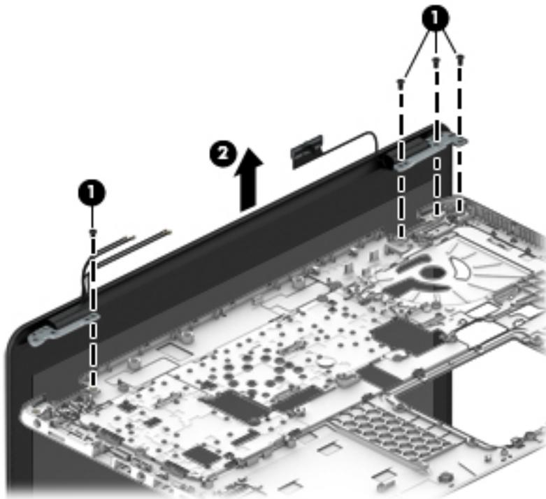
5. Lift the display assembly straight up and remove it (2).
