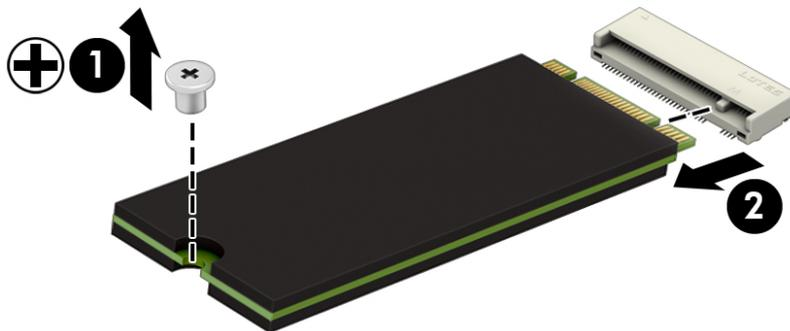
2. Remove the drive **(2)** by pulling it away from the connector.
