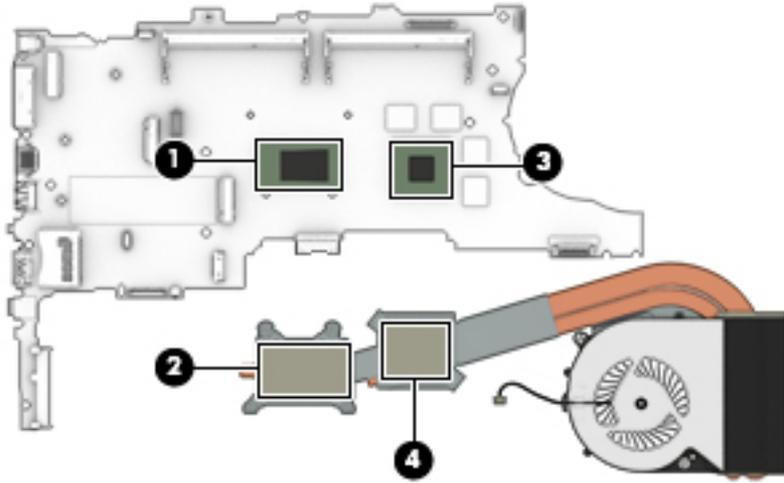
Reverse this procedure to install the heat sink/fan assembly.
