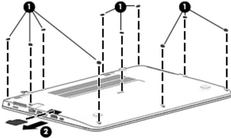
3. Remove the screws that secure the bottom cover to the computer.
