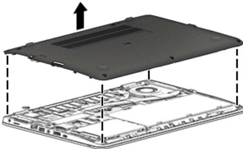
Reverse the removal procedures to install the bottom cover.
