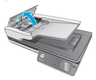
3. Squeeze the tabs on the sides of the roller cover, and then lift it up the roller cover to remove.
