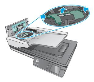
4. Remove and replace the rollers as described in the instructions included with the replacement kit.
