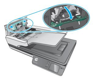
2. Remove the roller shaft from the holder, and then remove the roller module.
