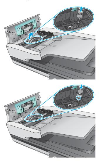
5. Replace the roller cover, and then continue with replacing the pick up roller module.
