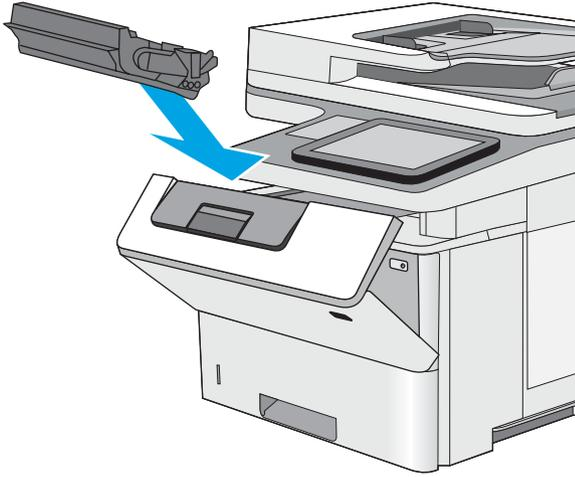
**EN** Align the toner cartridge with the tracks inside the printer, and install the toner cartridge until it is firmly seated.
