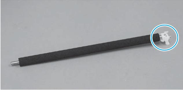
**EN** Remove the clip from the right end of the transfer roller. Set the clip aside, it will be installed on the replacement roller.
