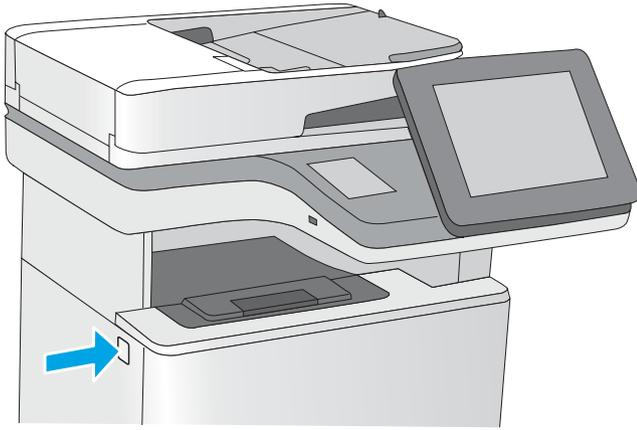
**EN** Press the cartridge-door-release button.
