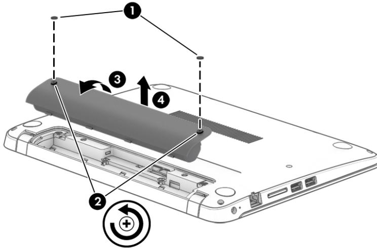
Reverse this procedure to install the battery.
