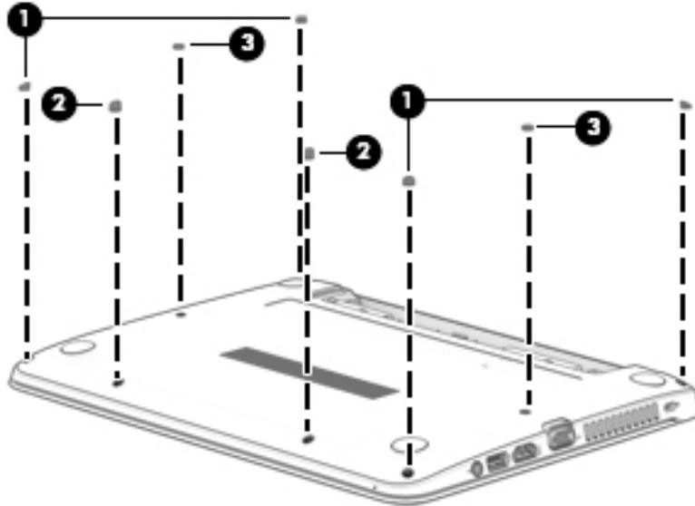
2. Remove the eight Torx T8M2.0×5.6 screws **(4)** that secure the bottom cover to the computer.
