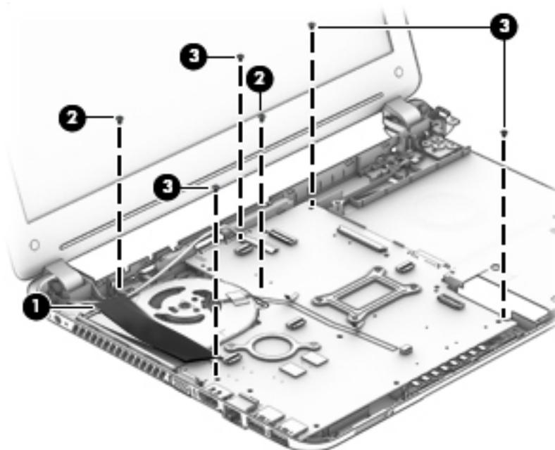
8. Carefully flex the right side of the base enclosure **(1)** so that the connectors on the right side of the system board clear the base enclosure.
