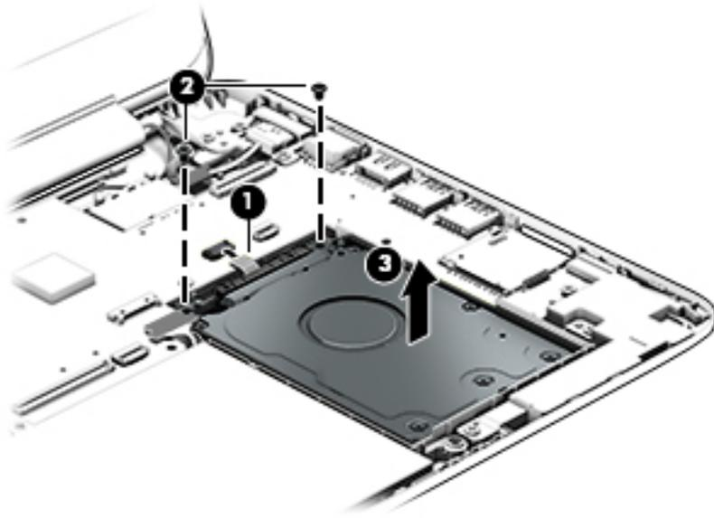
4. If it is necessary to replace the hard drive bracket, remove the four Phillips PM3.0×4.1 screws (1) that secure the hard drive bracket to the hard drive.
