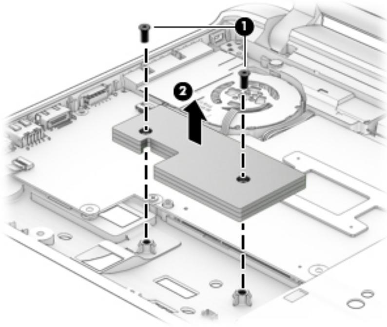
Reverse this procedure to install the counterweight.
