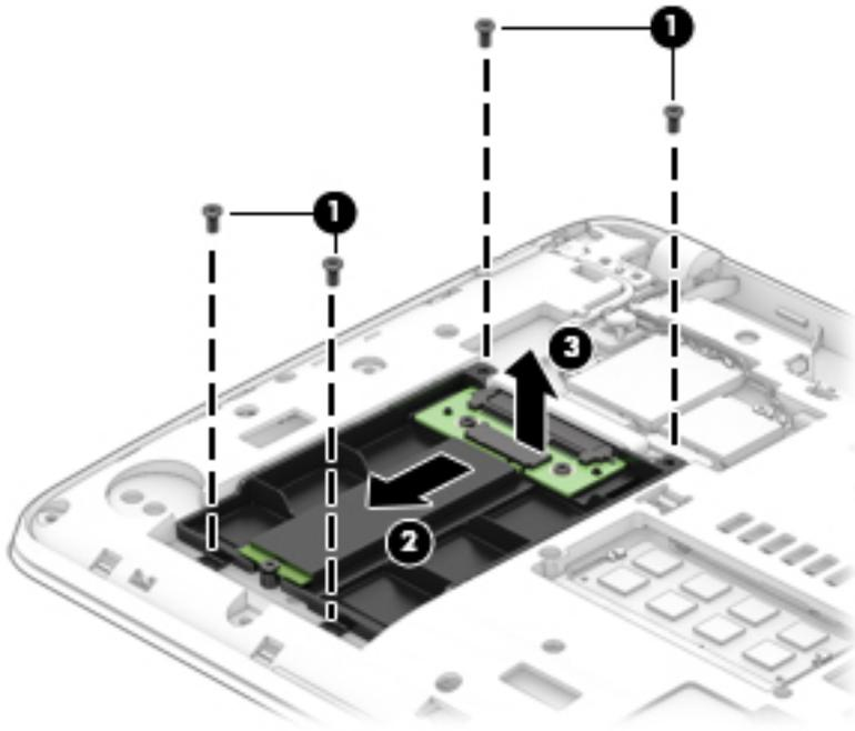
6. If it is necessary to replace the solid-state drive connector board, remove the two Phillips PM2.0×3.7 broad head screws (1) that secure the solid-state drive connector board to the solid-state drive tray.
