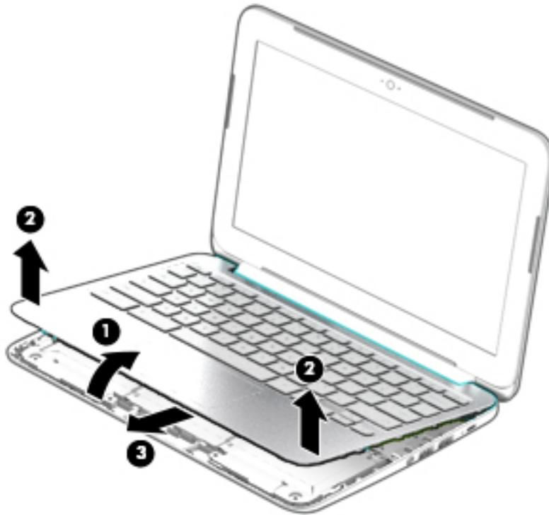
Reverse this procedure to install the keyboard/top cover.
