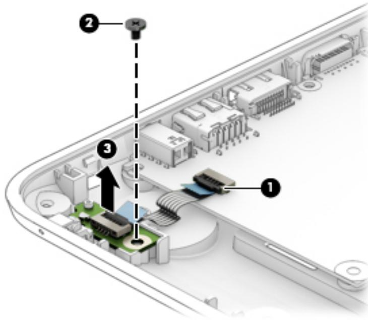
Reverse this procedure to install the hard drive LED board.
