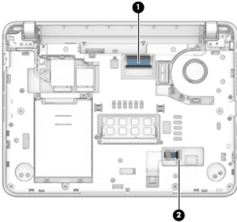
3. Remove the following screws that secure the keyboard/top cover to the base enclosure:
