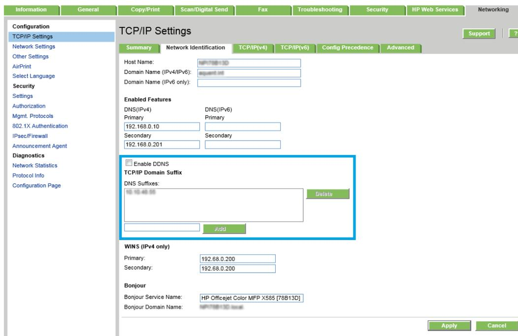
The screenshot shows the 'TCP/IP Settings' dialog box with the 'Network Identification' tab selected. The 'Enable DDNS' checkbox is checked. The 'TCP/IP Domain Suffix' section is highlighted with a blue box, showing a list of DNS suffixes with 'Add' and 'Delete' buttons. Below it, the 'WINS (IPv4 only)' and 'Bonjour' sections are visible.
