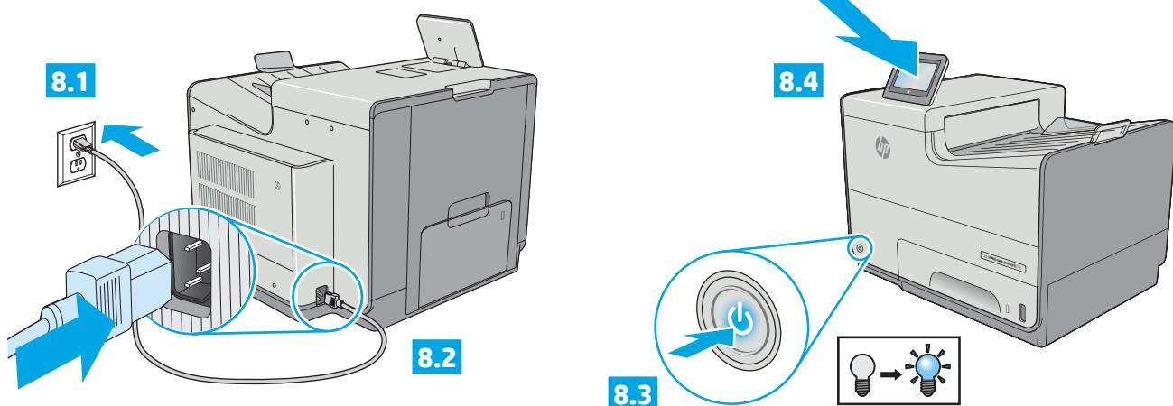
**EN** Connect the power cable between the product and a grounded AC outlet. Turn on the product. On the control panel, set the language, the keyboard layout, the date/time format, and the time zone. Allow the product to set up before printing, which will take some time. When the Home screen appears, touch **Initial Setup**, and enable basic product functions.
