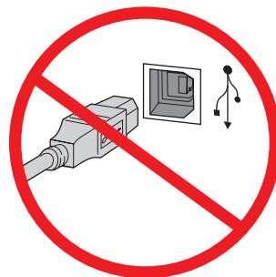
**EN** **Windows:** Do not connect the USB cable until prompted during the software installation in the next step. If the network cable was connected in step 7, proceed to step 10.
