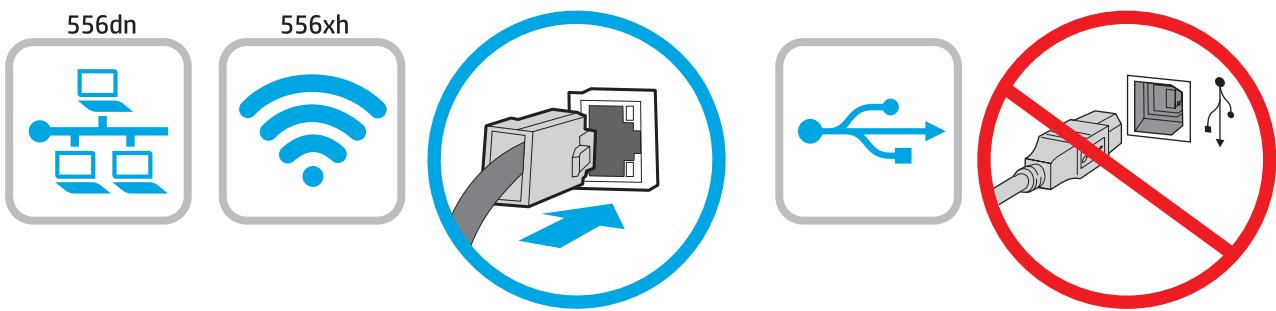
**EN** If you are connecting to a network, connect the network cable now. **CAUTION:** Do not connect the USB cable now.
