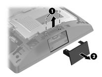
Insert the USB connector on the fingerprint reader into the side USB port ①, and then secure the module with the two screws that were previously removed ②.
