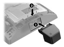
4. Align the tabs on the display head rear cover with the slots on the display head. Place the cover on the display head, and then slide the cover down so that it snaps in place.
