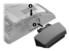
Align the tabs on the display head rear cover with the slots on the display head. Place the cover on the display head, and then slide the cover down so that it snaps in place.
