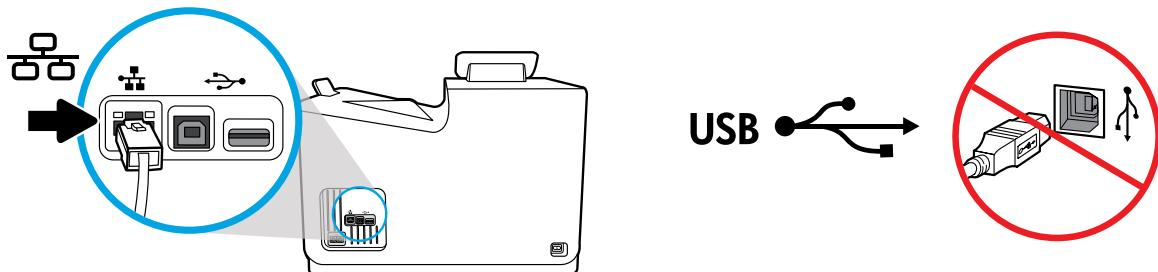
**EN** Connect Ethernet cable, if you want Ethernet connection to network. **Do not connect USB cable at this time.**
