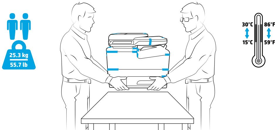
**EN** Place printer in sturdy, well-ventilated, dust-free area, away from direct sunlight. Keep printer level to avoid cartridge leakage. Printer and ambient temperature should be 15°-30° C (59°-86° F).
