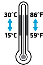
**EN** Place printer in sturdy, well-ventilated, dust-free area, away from direct sunlight. Keep printer level to avoid cartridge leakage. Printer and ambient temperature should be 15°-30° C (59°-86° F).
