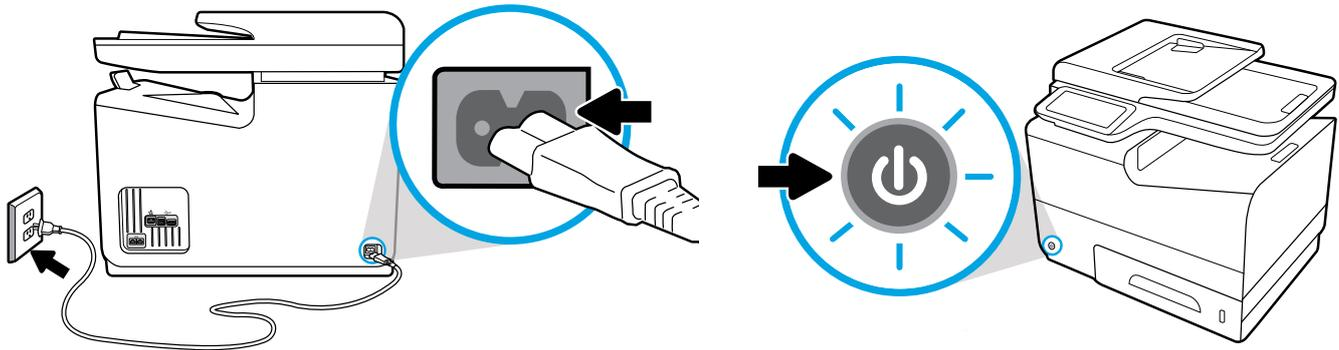
**EN** Connect power cord to ac outlet. Turn on printer.
