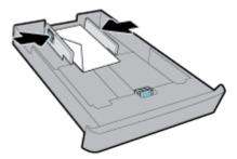
**6.** Make sure the stack of envelopes does not exceed the stack height marking on the left paper-width guide.
