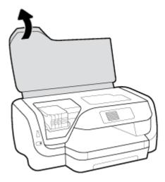
**2.** If the print carriage is not obstructed, move the print carriage to the rightmost end, and remove the jammed paper with both hands.
