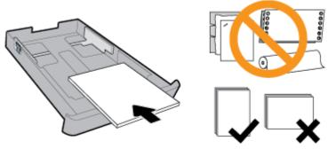
Make sure the stack of paper is aligned with the appropriate paper size lines on the front of the tray. Besides, make sure the stack of paper does not exceed the stack height marking on the right edge of the tray.
