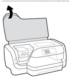
**ENWW** Replace the cartridges 39 **3.** Press the front of the cartridge to release it, and then remove it from the slot.
