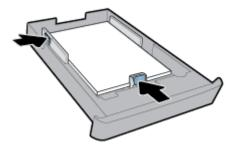
**5.** Reinsert the input tray back into the printer.
