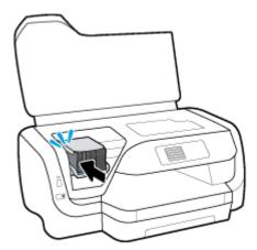
Make sure that the color on the cartridge matches the color on the slot.
