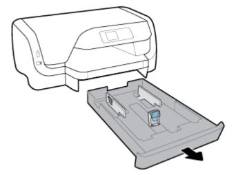
**2.** Check the gap under the printer where the input tray was. Reach into the gap and remove the jammed paper.
