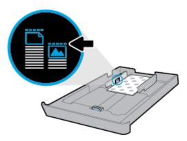
7. Adjust the paper-length guide until it touches the edge of the stack of paper.
