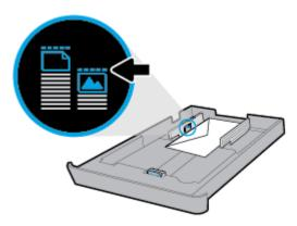
7. Adjust the paper-length guide until it touches the edge of the stack of envelopes.
