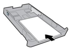
Make sure the stack of paper is aligned with the appropriate paper size lines on the front of the tray. Besides, make sure the stack of paper does not exceed the stack height marking on the right edge of the tray.
