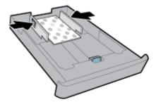
**6.** Make sure the stack of paper does not exceed the stack height marking on the left paper-width guide.
