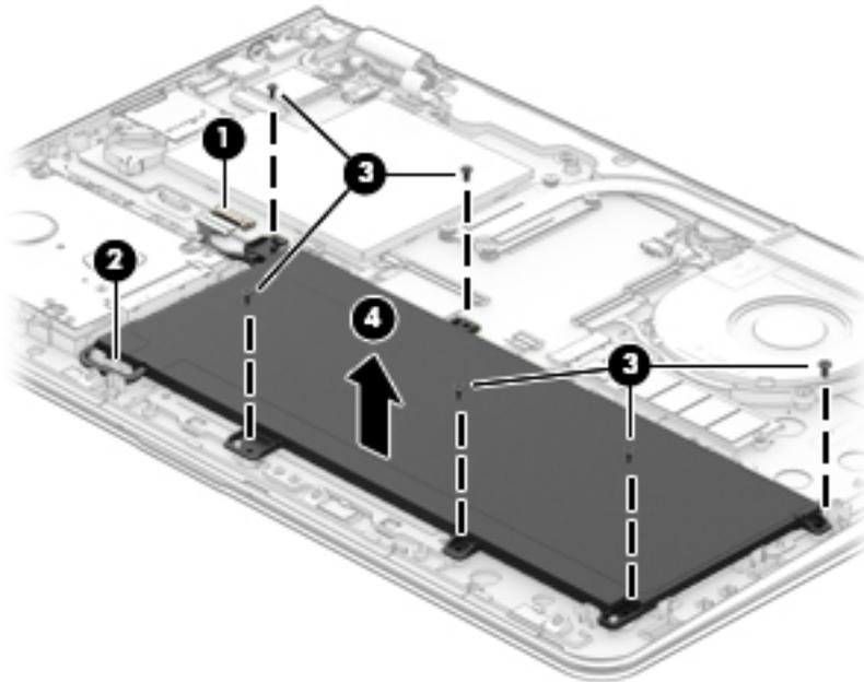
Reverse this procedure to install the battery.
