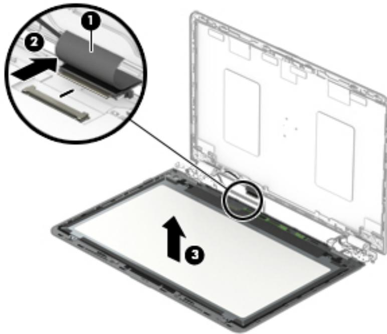
6. If it is necessary to replace the TouchScreen board cable:
