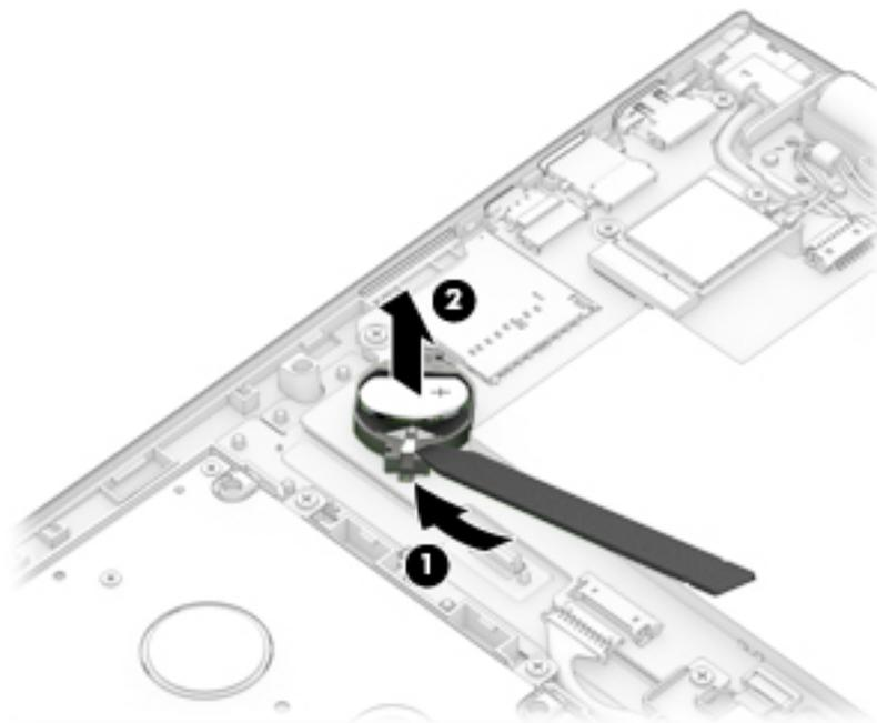
Reverse this procedure to install the RTC battery. When installing the RTC battery, make sure the “+” sign is facing up.
