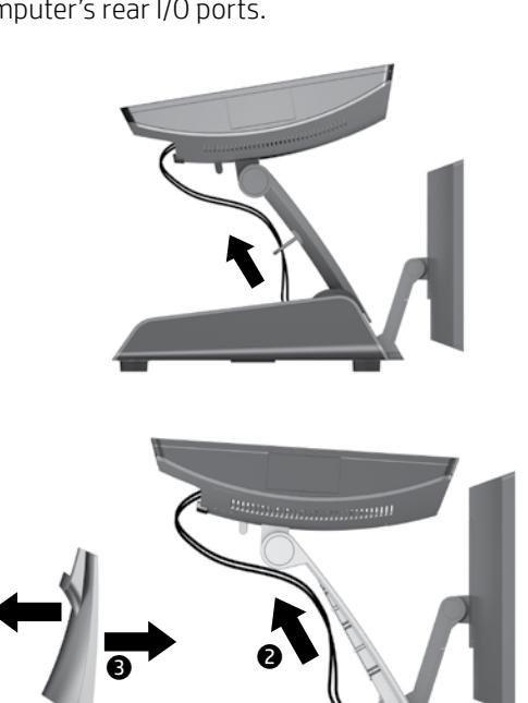
• If your retail system computer has an HP Compact Stand, remove the cable routing cover • from the stand, route the cables up and through the cable retainer clip • onto the stand, and then replace the cable routing cover • onto the stand to hide the cables.
