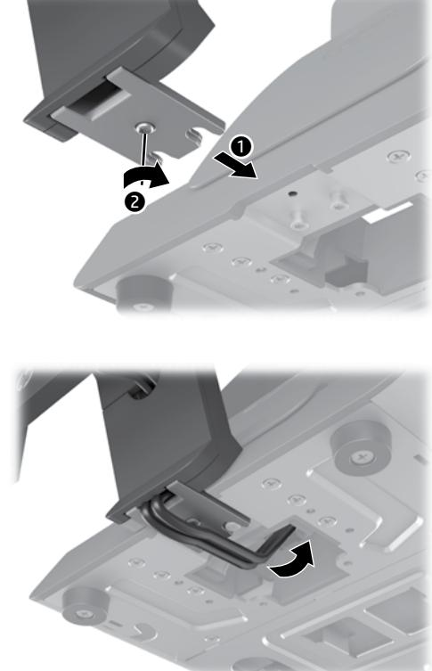
4 Thread the cables up and through the routing system on the stand model selected for your retail system computer, and then connect the cables to the retail system computer's rear I/O ports.
