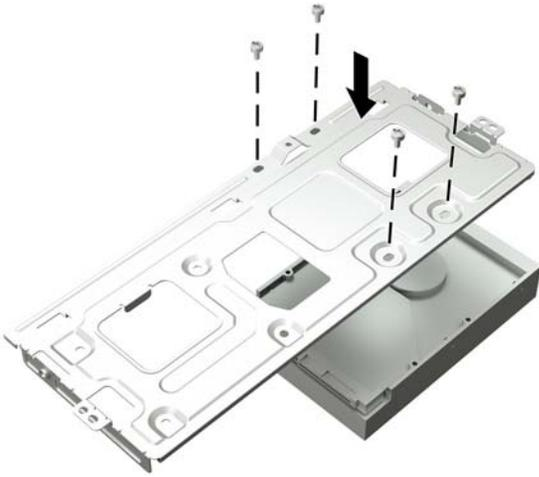
2. Position the drive cage perpendicular to the computer and insert the cage into the slots in the computer. Rotate the cage into place (1), and then slide the cage toward the front of the computer (2). Replace the three Phillips screws (3).
